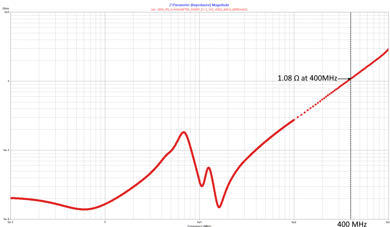
Figure 3-1. VDDS_MMC0 AC Impedance Magnitude vs Frequency (Board Only)
