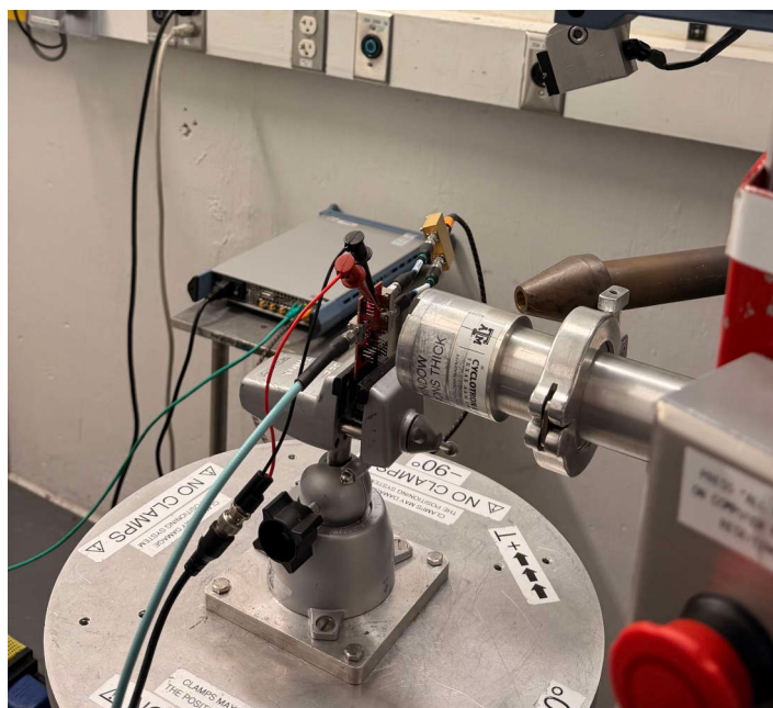
Figure 4-1. Decapped TRF0108-SP Evaluation Board Mounted in Front of the Heavy-Ion Beam Exit Port
