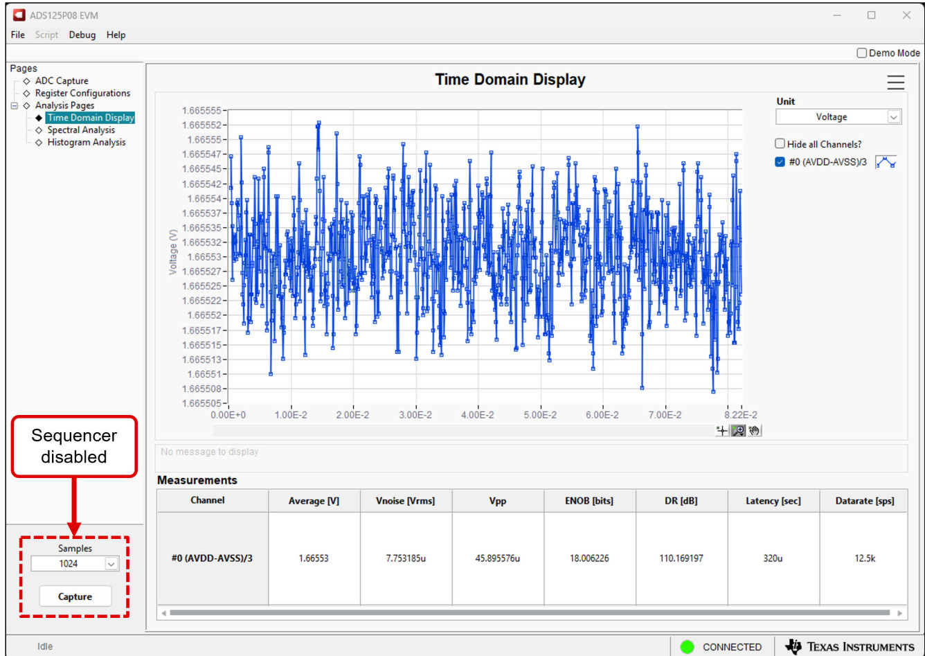
Figure 4-8. ADS125P08 EVM GUI Time Domain Page - Sequencer Disabled
