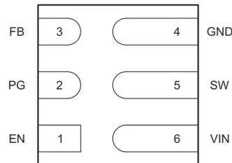
Figure 5-1. DMQ Package, 6-Pin VSON-HR (Bottom View)
