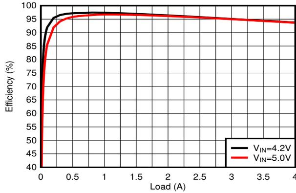
$V_{OUT} = 3.3V$  F-PWM devices
