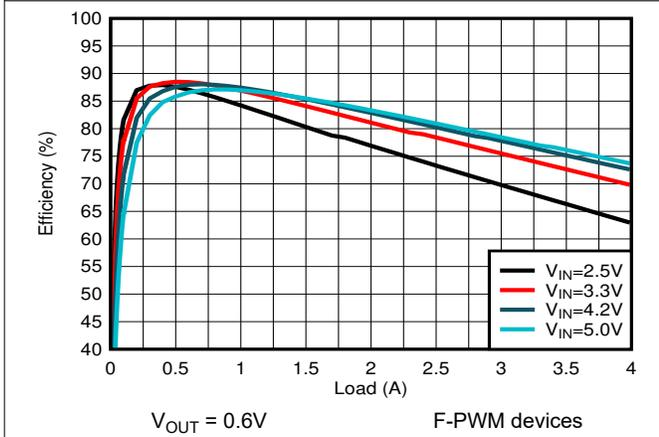
Figure 8-5. PWM Efficiency
