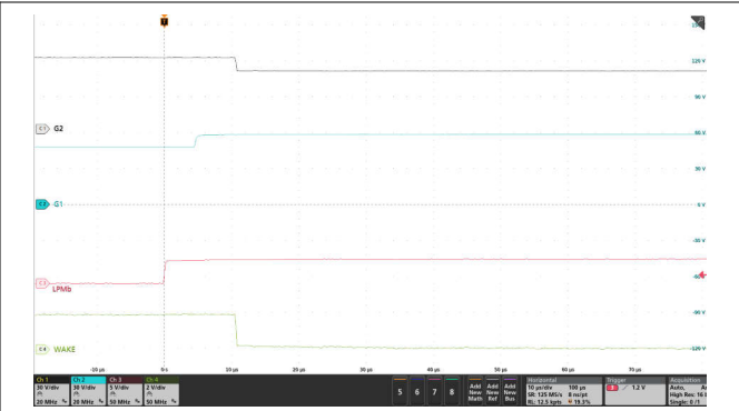
Figure 8-5. State Transition From LPM to Active Mode ( \overline{\text{LPM}} = \text{Low to High} , V_{\text{IN}} = 48\text{V} , No Load)
