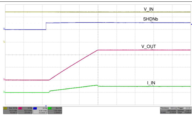
Figure 57. Start-Up With VIN—No Load
