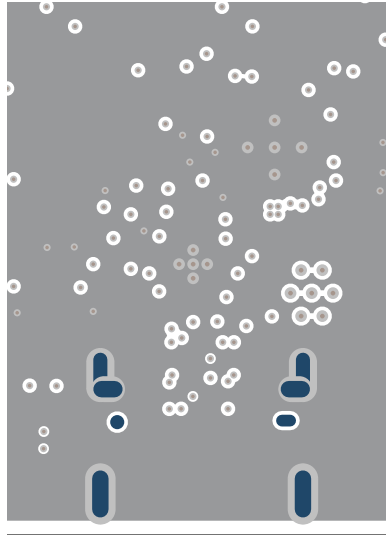
Figure 7-9. TPS26750 PCB Layout - GND Layer 5
