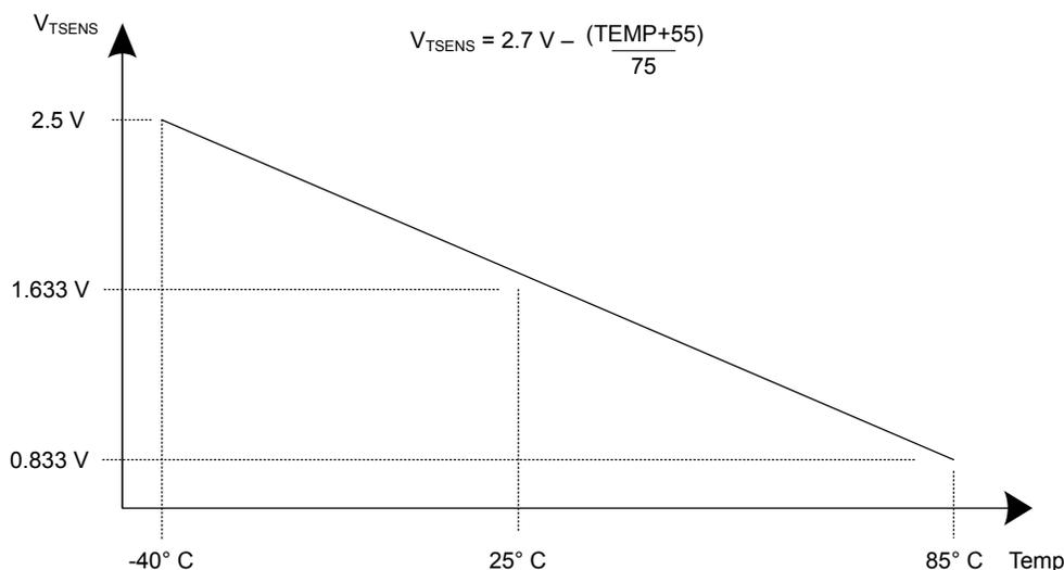
The temperature sensor reading can be sampled in a sample sequence by setting the  $TS_n$  bit in the **ADCSCTLn** register. The temperature reading from the temperature sensor can also be given as a function of the ADC value. The following formula calculates temperature (TEMP in °C) based on the ADC reading ( $ADC_{CODE}$ , given as an unsigned decimal number from 0 to 4095) and the maximum ADC voltage range ( $V_{REFP} - V_{REFN}$ ):
