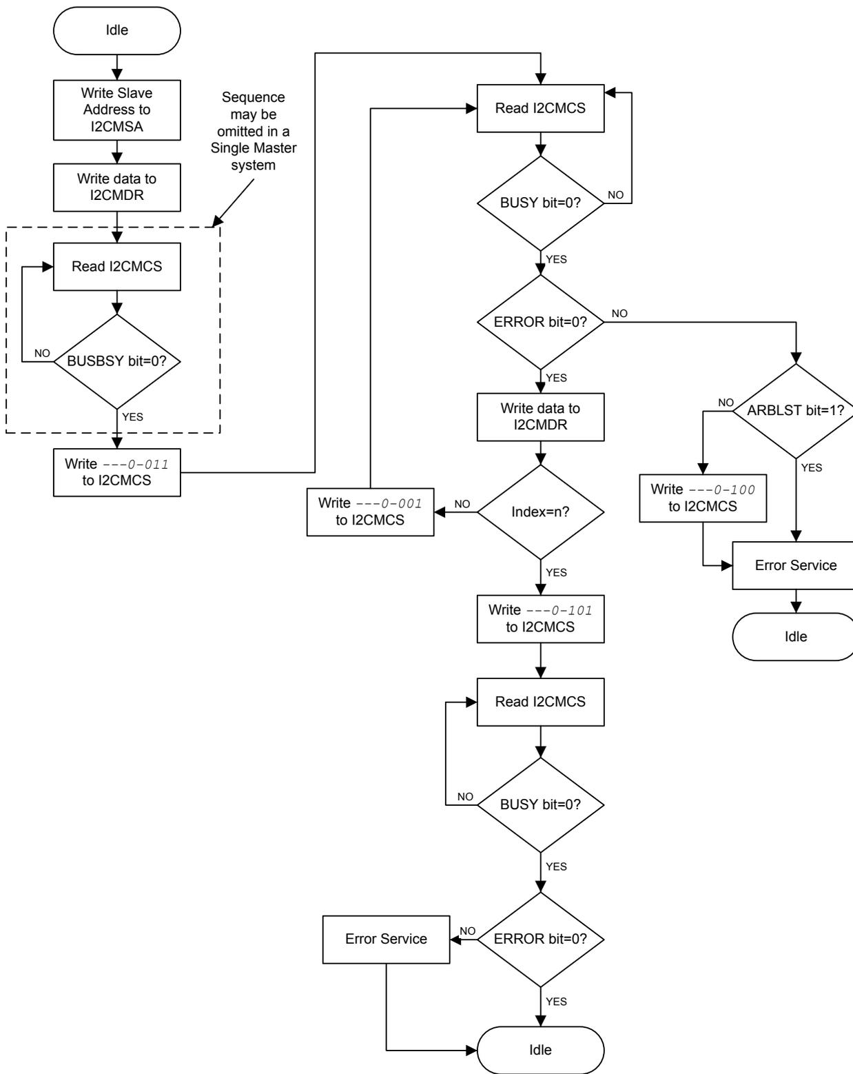
Figure 15-11. Master RECEIVE of Multiple Data Bytes
