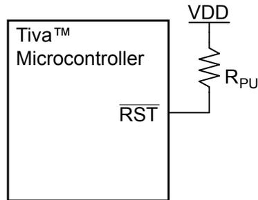
$R_{\text{PU}} = 0$  to 100 k $\Omega$
