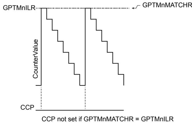
Figure 10-8 on page 652 shows how the CCP output operates when the `PLO` and `MRSU` bits are set and the `GPTMTnILR` is greater than the `GPTMTnMATCHR` value.
