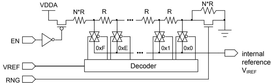
**Note:** In the figure above,  $N \cdot R$  represents a multiple of the  $R$  value that produces the results specified in Table 18-2 on page 1148.
