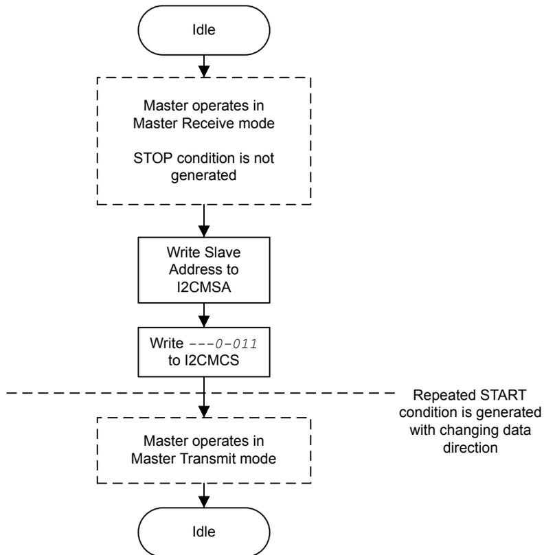
Figure 15-14. Standard High Speed Mode Master Transmit
