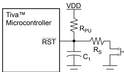
Typical  $R_{PU} = 10\text{ k}\Omega$
