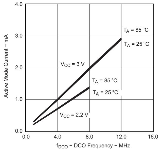
Figure 3. Active Mode Current vs DCO Frequency
