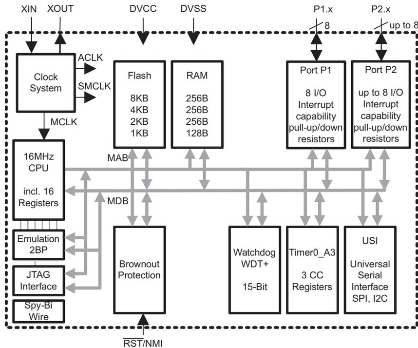
NOTE: Port P2: Two pins are available on the 14-pin and 16-pin package options. Eight pins are available on the 20-pin package options.
