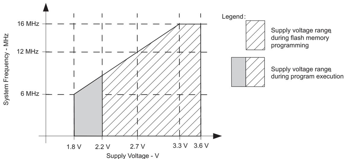
Note: Minimum processor frequency is defined by system clock. Flash program or erase operations require a minimum V<sub>CC</sub> of 2.2 V.
