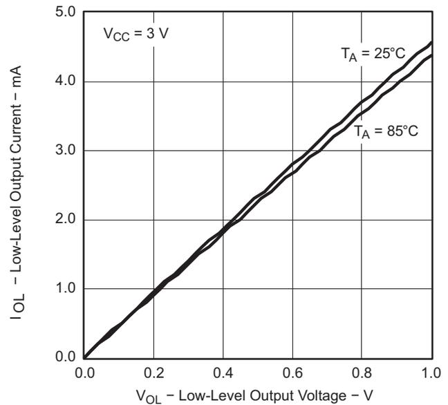
Figure 17. USI Low-Level Output Voltage vs Output Current
