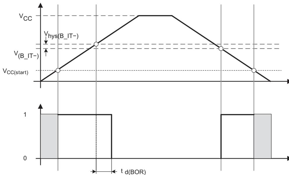
Figure 12. POR and BOR vs Supply Voltage
