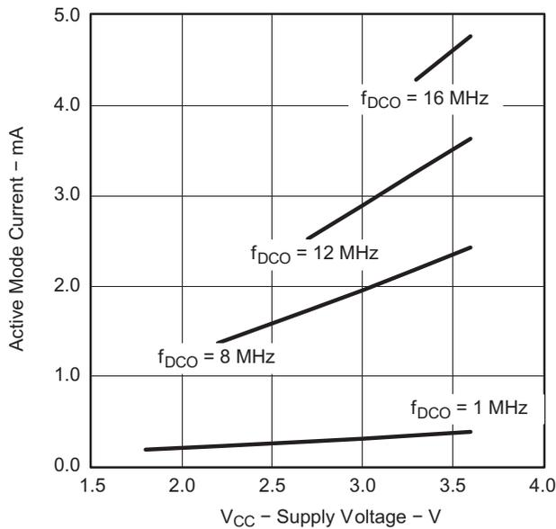
Figure 2. Active Mode Current vs  $V_{CC}$ ,  $T_A = 25^\circ\text{C}$
