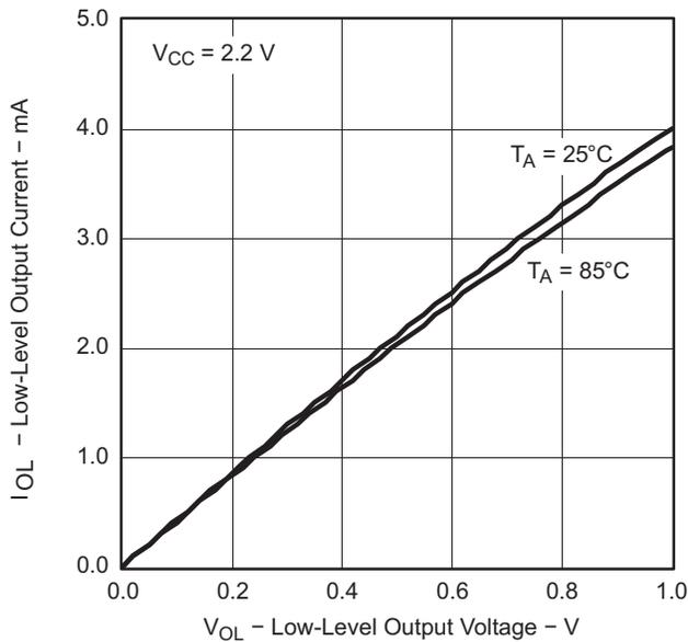
Figure 16. USI Low-Level Output Voltage vs Output Current
