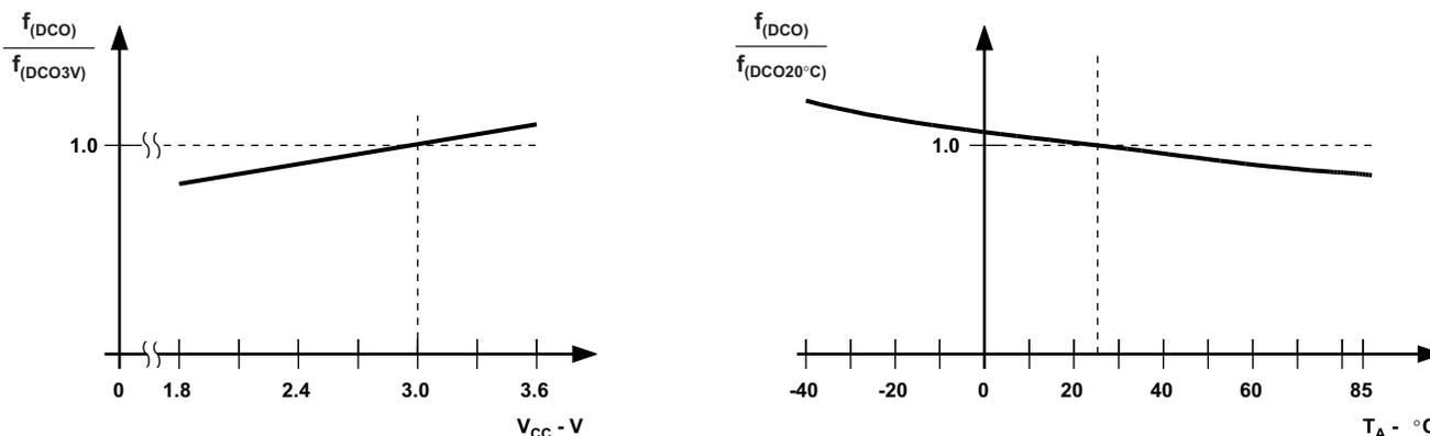
Figure 5-15. DCO Frequency vs Supply Voltage V<sub>CC</sub> and vs Ambient Temperature
