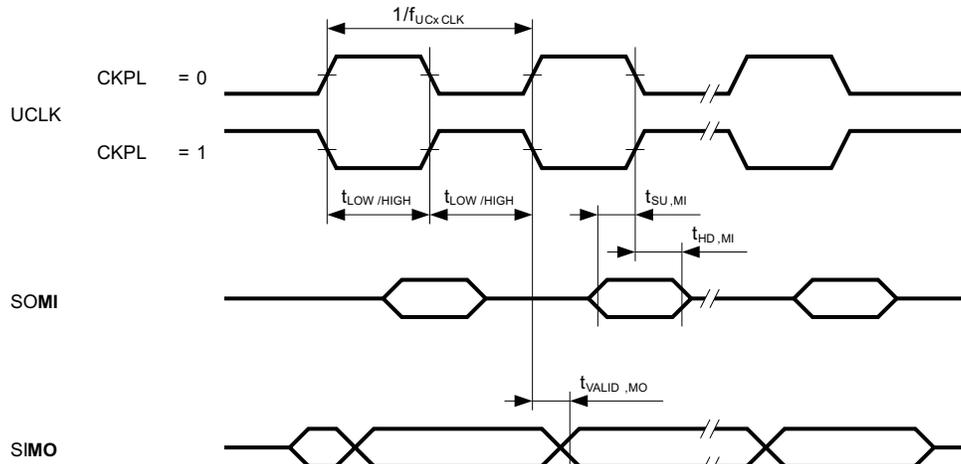
Figure 5-18. SPI Master Mode, CKPH = 0
