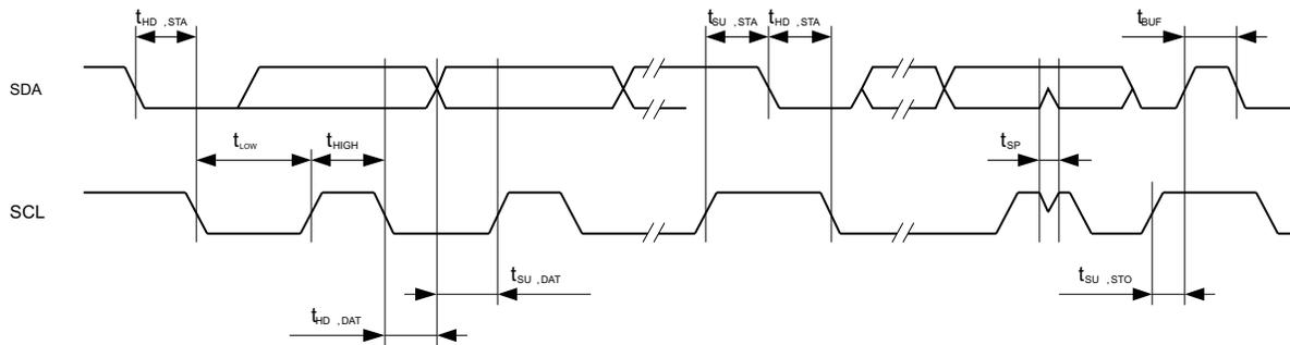
Figure 5-22. I<sup>2</sup>C Mode Timing
