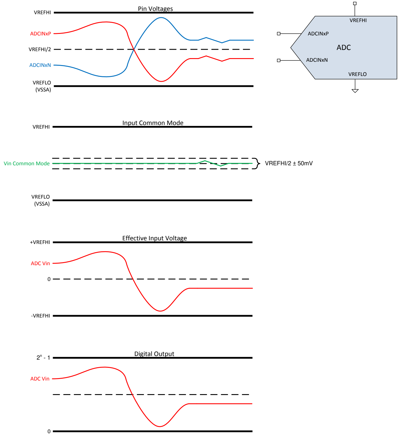
Figure 6-36. Differential Signaling Mode
