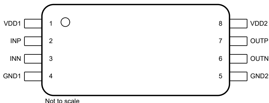
Figure 5-1. DWL Package, 8-Pin SOIC (Top View)
