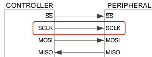
**SCLK** is the SERIAL CLOCK. As mentioned previously, SCLK is used by the controller to synchronize the data sent between the controller and the peripheral device. The SCLK originates from the controller and is sent to all peripheral devices. This serial clock may not always be in operation, and may be idle as a high or low signal. Data is clocked into the controller or peripheral at either the rising edge or falling edge of the serial clock. The SCLK line may also be labeled as SCK.
