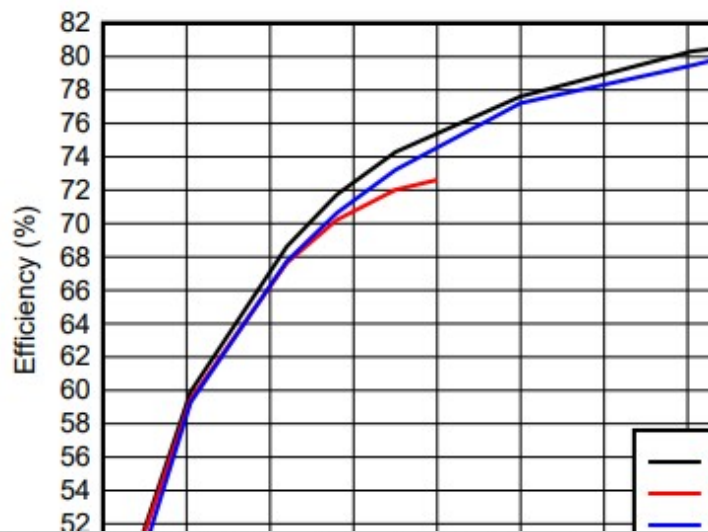
Measured Efficiency Under Input Voltages of 5V, 12V, and 18V
