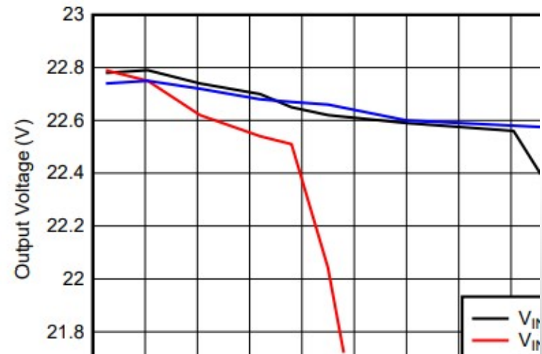
Load Regulation Under Input Voltages of 5V, 12V, and 18V
