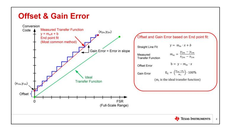
Let's start with the basic calculation for offset and gain error. The key to understanding this is to know that the ADC transfer function is not perfectly linear, so a linear curve fit is applied to the function. For this calculation, the most commonly used type of curve fit is an end point linear fit. With this type of curve fit, the first and last points on the ADC transfer function define the straight line.
