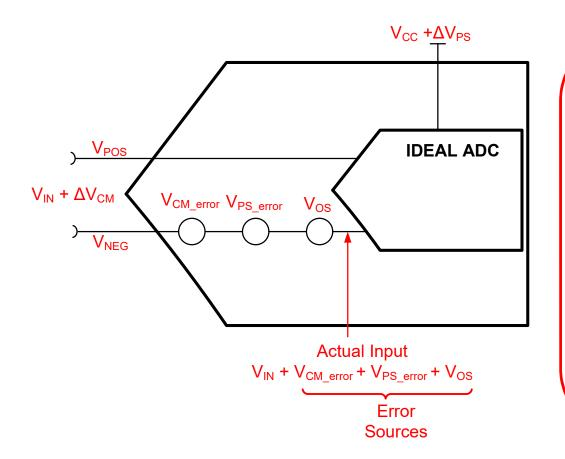
$$V_{CM} = \left(\frac{V_{POS} + V_{NEG}}{2}\right)$$
