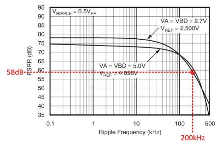
$$\Delta V_{PS\_error} = \Delta V_{PS} \cdot 10^{\left[\frac{-PSR (dB)}{20}\right]}$$
