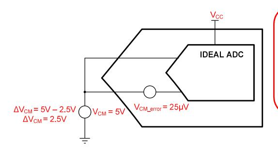
$$V_{CM} = \left(\frac{V_{POS} + V_{NEG}}{2}\right)$$
