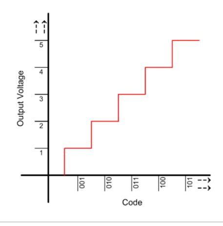
**Resolution** = n – The number of bits used to quantify the output
