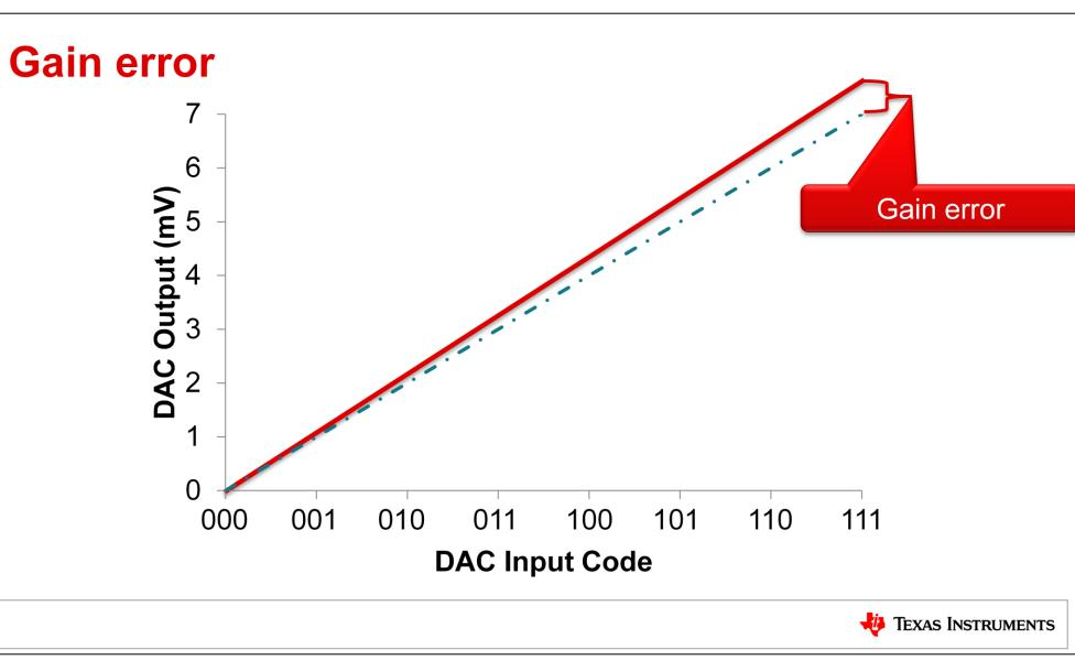
The next specification to consider is **gain error**. If offset error is the b term in y = mx + b then gain error can be considered the m term. Gain error describes the deviation from the ideal slope of the transfer function defined as 1 LSB. Similar to offset error, this is based on a line of best fit taken from a two-point measurement of the DAC output.
