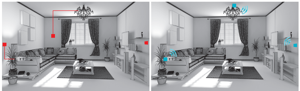
Figure 5. Light switch (a) in the traditional way and (b) IoT-enabled
