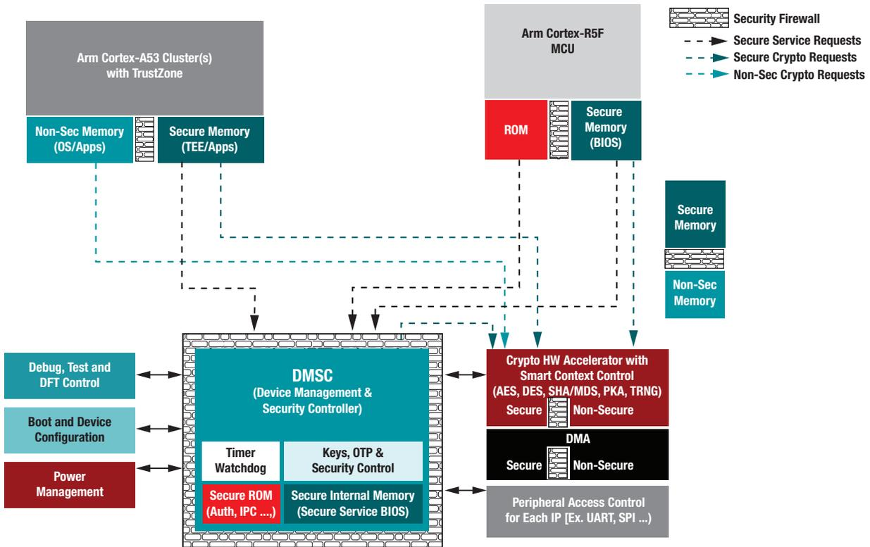
Figure 3: DMSC features integrated on AM6x processors.
