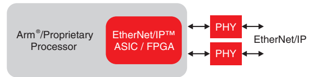
Figure 8. Integrated EtherNet/IP with processor.
