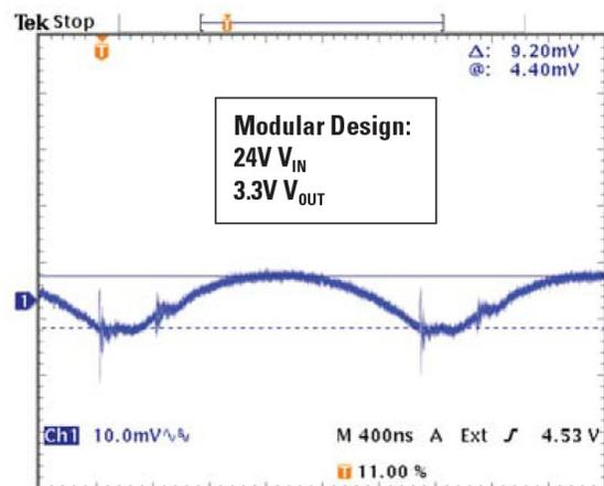
Note: AC-coupled output noise. BW = 150 MHz. Very low inductance probe across output capacitors.
