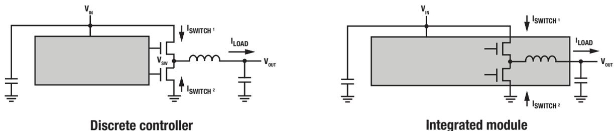
Figure 1. DC-DC buck regulator integration levels.
