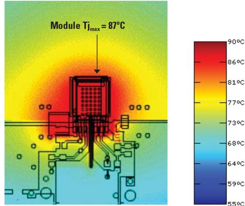
Figure 7. WEBENCH simulation output for a modular design.
