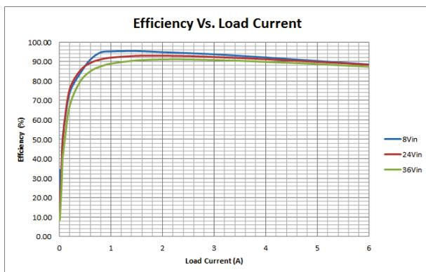
**Figure 7.** LMZM33606 efficiency.
