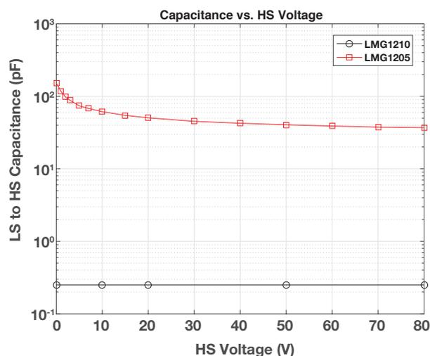
**Figure 3.** High-side to low-side capacitance vs. voltage
