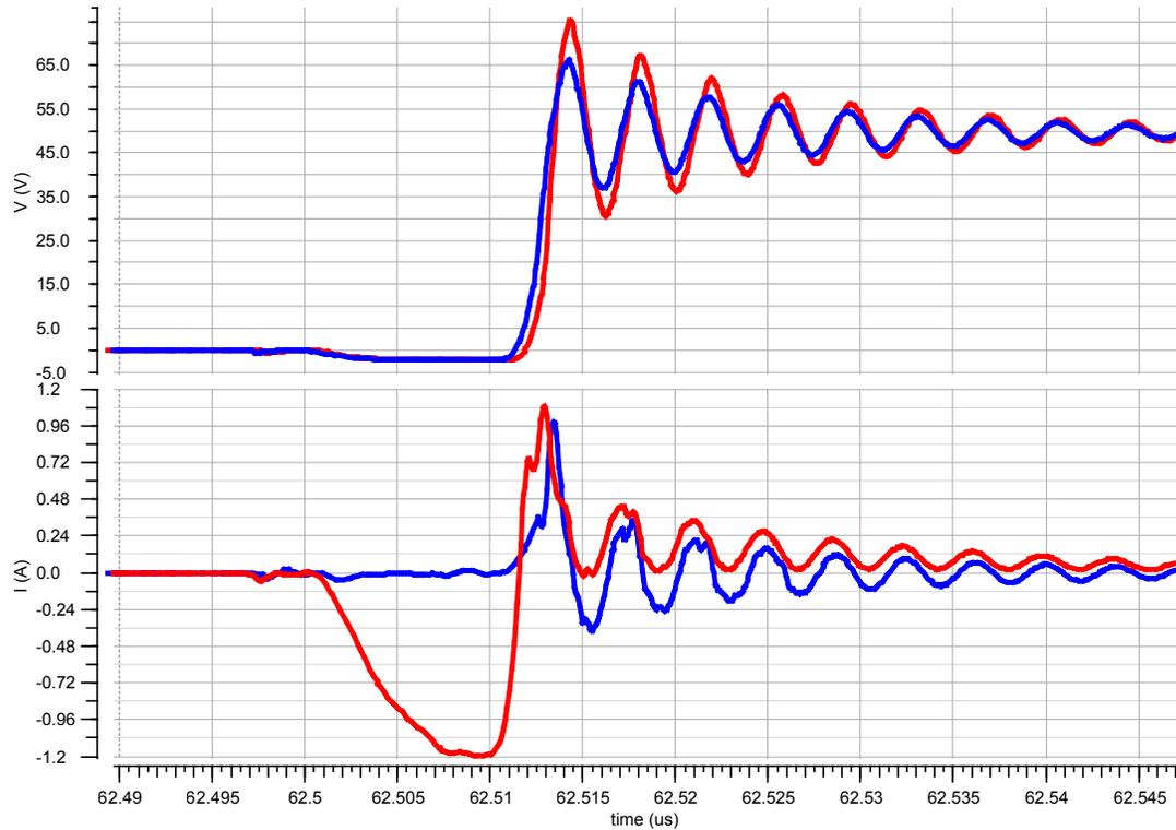
**Figure 2.** Switch-node voltage (top) and bootstrap current (bottom). The red line is the LMG1205 style showing a surge of current right before the diode reverses. The blue line is the LMG1210 style where the bootstrap shuts off before the dead time.
