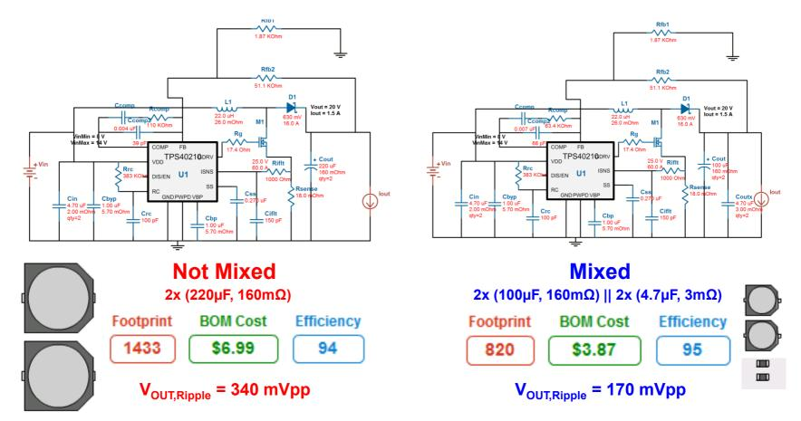
Mixed-cap design (24 components, 21 unique) results in **42% smaller footprint, 44% lower cost**, and **50% smaller output ripple than nonmixed design** (22 components, 20 unique)
