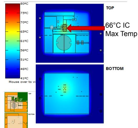
Lower temperature leads to better reliability. Thermal simulations allow designer to make the tradeoff of reliability with footprint.
