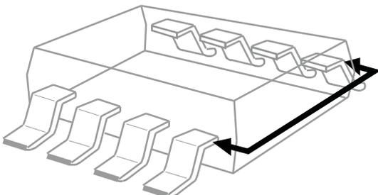
**Figure 2.** Illustration of creepage.
