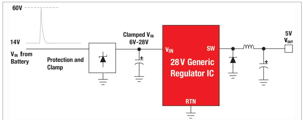
Figure 3a. A generic 24V regulator with in a battery-supplied system with voltage clamp for protection against input voltage surges.
