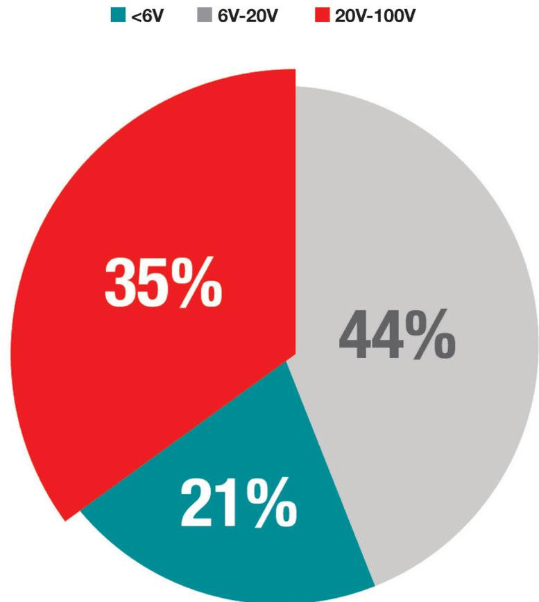
Figure 1. 35% of power management ICs (controllers and regulators) are rated above 20V.
