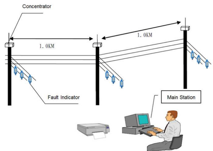
**Figure 2.** A smart fault indicator system
