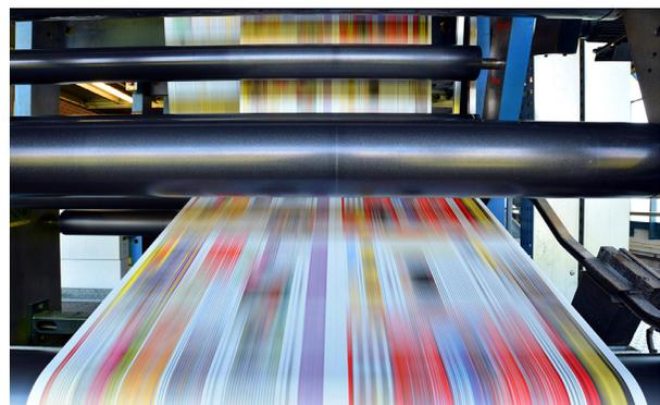
*Figure 3: Flexographic printing.*
