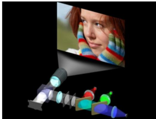
Figure 4. DMD in an LED-based optical system
