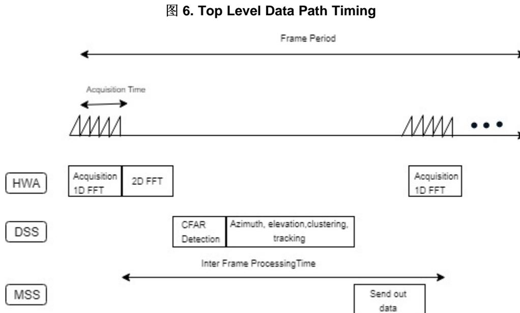
图 6 also shows the data path processing, which is described as follows.
