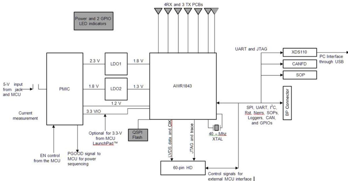
For more details on the hardware, see the [AWR1843 single-chip 76-GHz to 81-GHz automotive radar sensor evaluation module](#). The schematics and design database can be found in the following files: [AWR1843BOOST Design Database](#) and [AWR1843BOOST Schematic, Assembly, and BOM](#).
