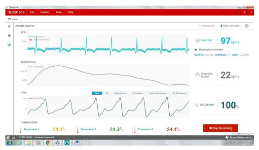
图 28. GUI Displaying ECG, Respiration and SPO2 Waveforms With SPO2 Number and Heart Rate
