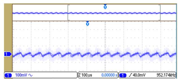
图 30. Output Ripple Voltage of 5.2 V Supply for Input Voltage of 3.7 V, and Input Current of 120 mA
