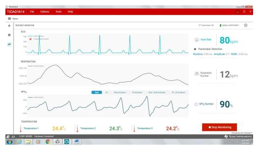
图 27. GUI Displaying ECG, SPO2 Waveforms With SPO2 Number and Heart Rate With ECG Sensitivity of 100-µVs
