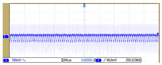
图 31. Output Ripple Voltage of 5 V Supply for Input Voltage of 3.7 V, and Input Current of 120 mA
