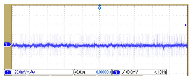
图 33. Output Ripple Voltage of 3.3 V Supply for Input Voltage of 3.7 V, and Input Current of 120 mA
