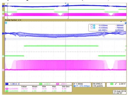
图 30. Valley Switching and ZVS Transition Zoom In (Channel 1: lin, Channel 3: GPIO)
