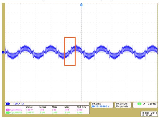
图 33. Input Current (Channel 1) Near Zero Crossing to Show the Control Logic Zoom In
