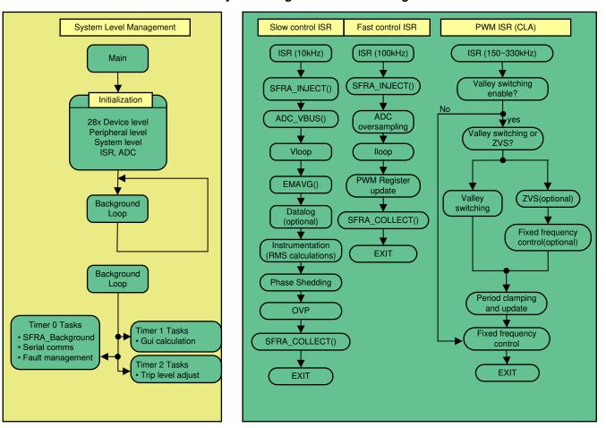
图 3. Valley Switching Firmware Flow Diagram
