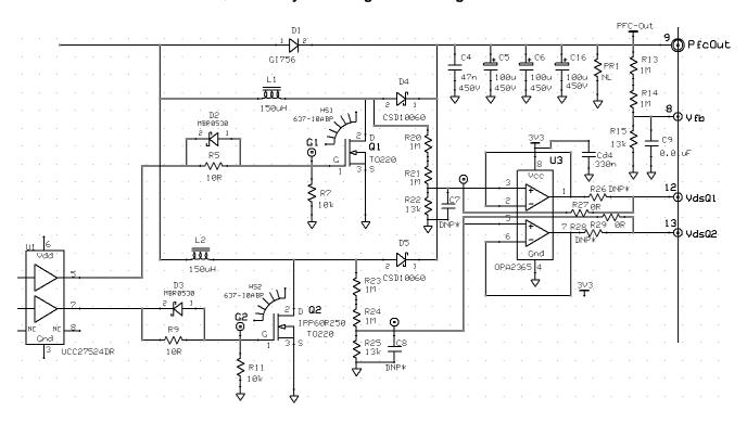
In this reference design, the valley switching schematic controlCARD interface is shown in 🛭 6. The Vds feedback paths are added based on the original ILPFC kit. Users do not need to connect both VdsQ1 and VdsQ2 to the controlCARD. If the phase 1 is working when valley switching is enabled, then only VdsQ1 is needed to feed back to the controlCARD which means only one voltage divider is needed in the circuit.
