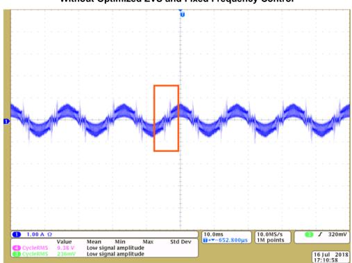
图 31. High Current Distortion Near Zero Crossing Point Without Optimized ZVS and Fixed Frequency Control
