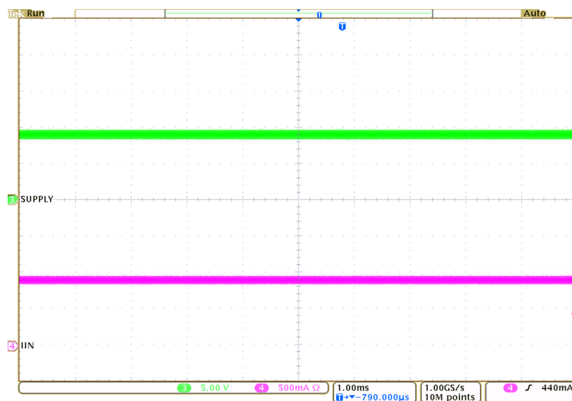
图 8. Operating Waveform, V_{IN} = 9\text{ V} CH3: Supply Voltage, CH4: Input Current
