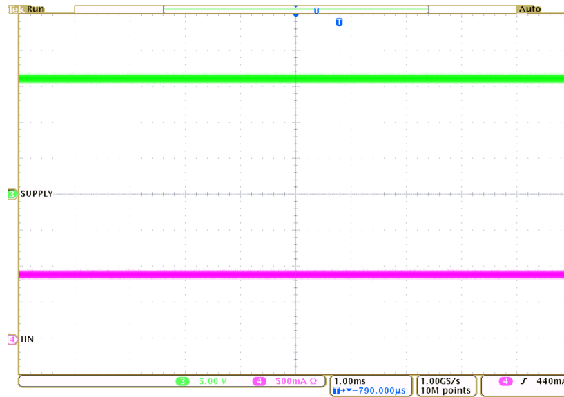
图 10. Operating Waveform, V_{IN} = 16\text{ V} CH3: Supply Voltage, CH4: Input Current
