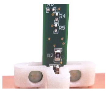
图 5. Zoomed-In Photo of Nylon Bolts Securing PCB
