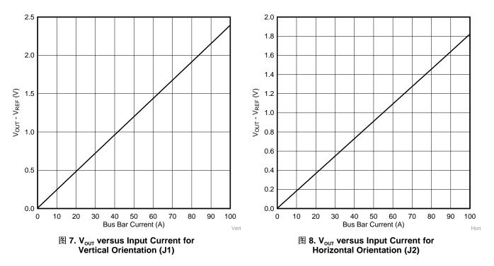
The gain and offset were calculated to increase accuracy. Calibrate the gain using 公式 1 for the vertical orientation and  ${\rm \ensuremath{\Delta x}}$  2 for the horizontal orientation. The offset is the measured  $V_{\text{out}}$  to  $V_{\text{REF}}$  when the current is 0 A.
