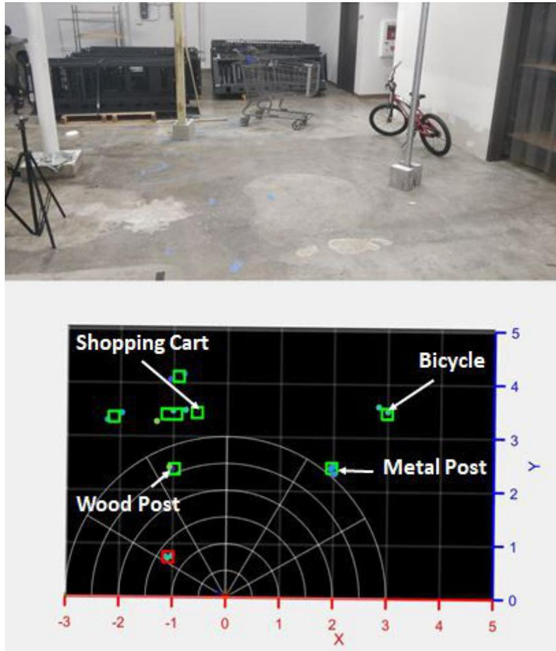
Figure 3-9. Multiple Object Detection
