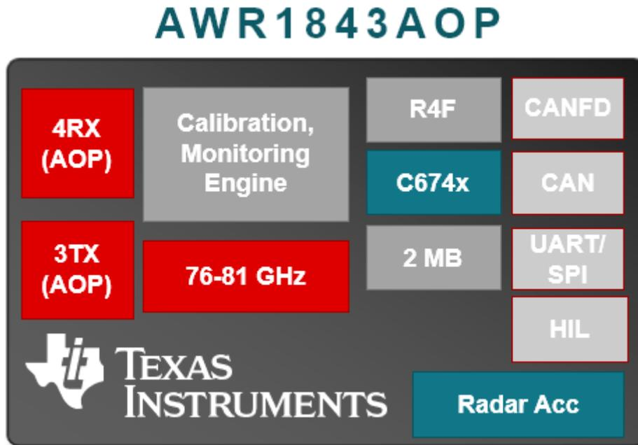
**Figure 2-2. AWR1843AOP Block Diagram**
