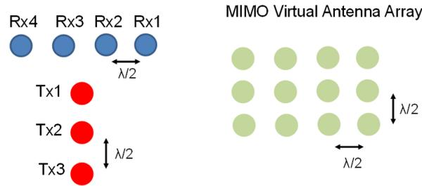
**Figure 2-3. AWR1843AOP-Antenna Pattern**
