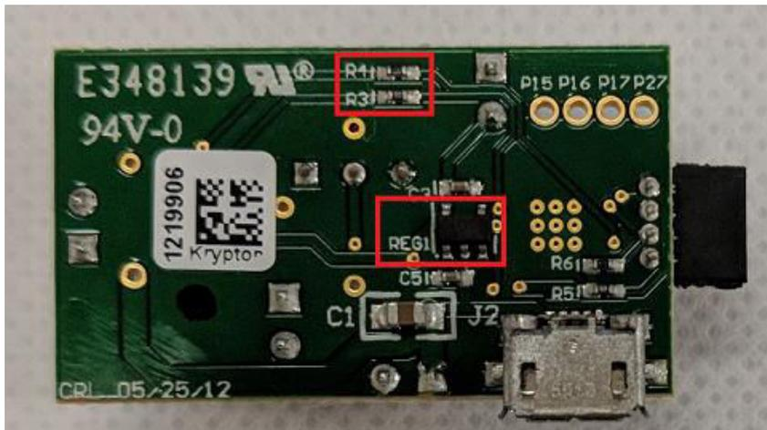
**Figure 3-13. Back of DRV8837EVM With Components To Remove Highlighted**
