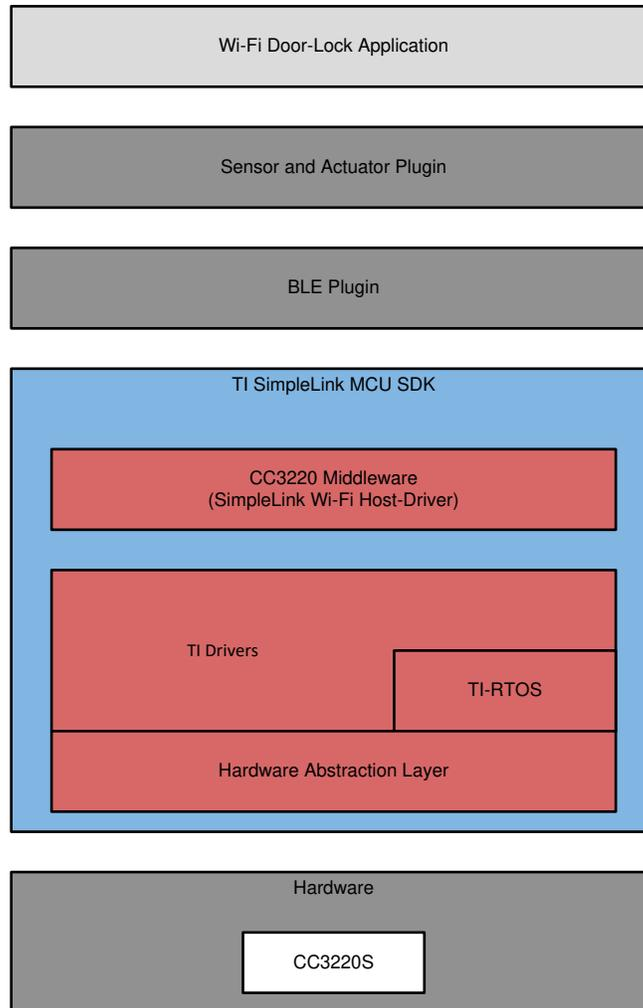
**Figure 2-3. Wi-Fi, Door-Lock Software Block Diagram**
