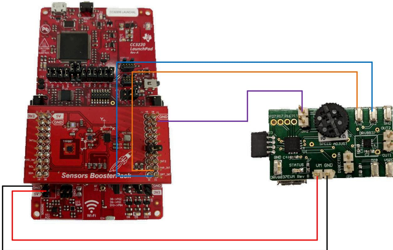
**Figure 3-6. Jumper Wire Placement to Connect DRV8837EVM to System**
