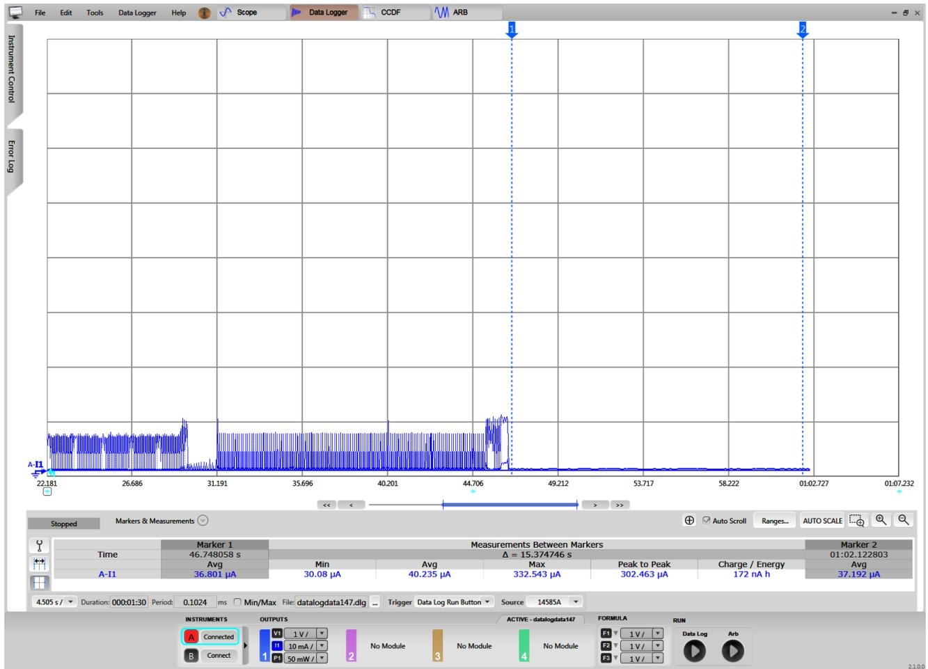
Figure 3-19. CC2640R2F Current Consumption While Idle
