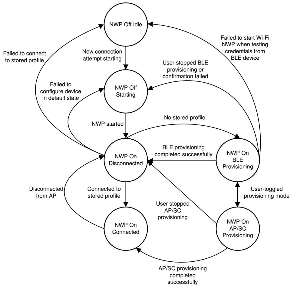
Figure 2-5. Network-Connection Management-Thread Flow Diagram
