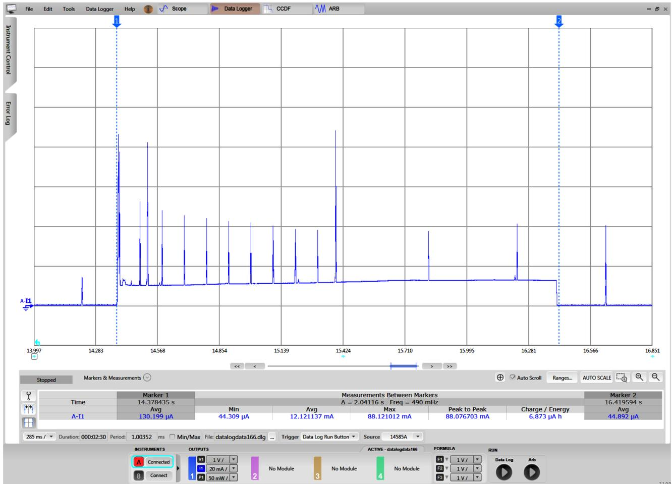
**Figure 3-16. CC3220 Current Consumption During Lock and Unlock Cycle**
