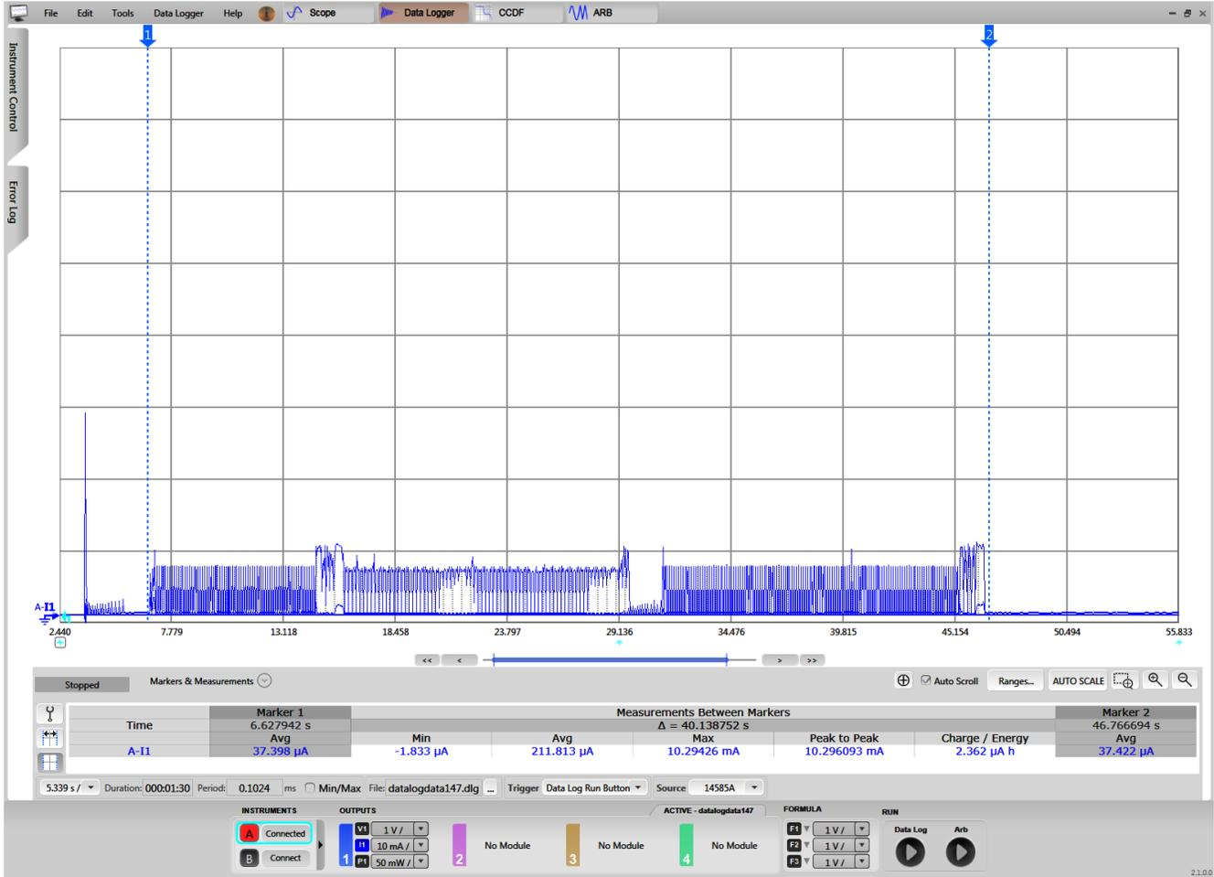
**Figure 3-18. CC2640R2F Current Consumption During Provisioning**
