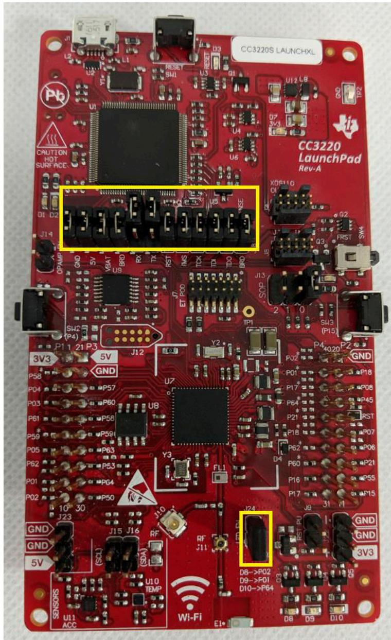
**Figure 3-1. CC3220S-LAUNCHXL Jumper Configuration**
