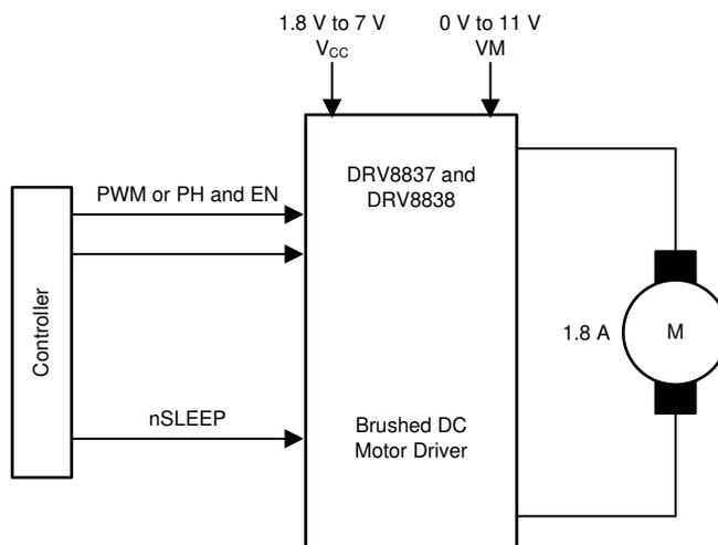
Figure 2-2. DRV8837 Simplified Diagram
