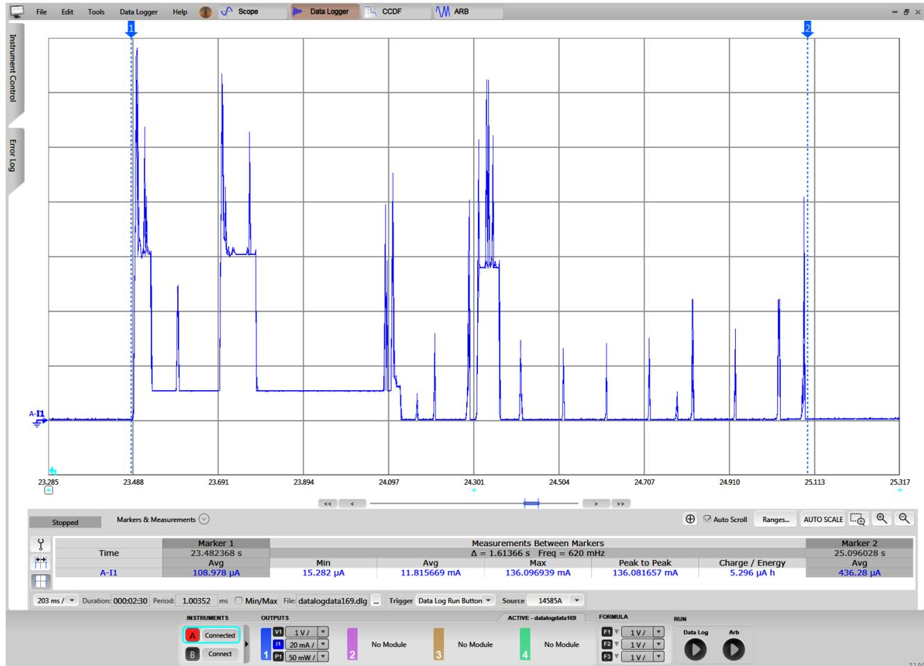
Figure 3-17. CC3220 Current Consumption During Lock Status Request
