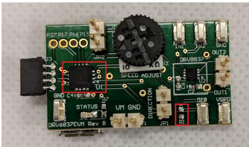
**Figure 3-14. Front of DRV8837EVM With Highlighted Components To Remove**
