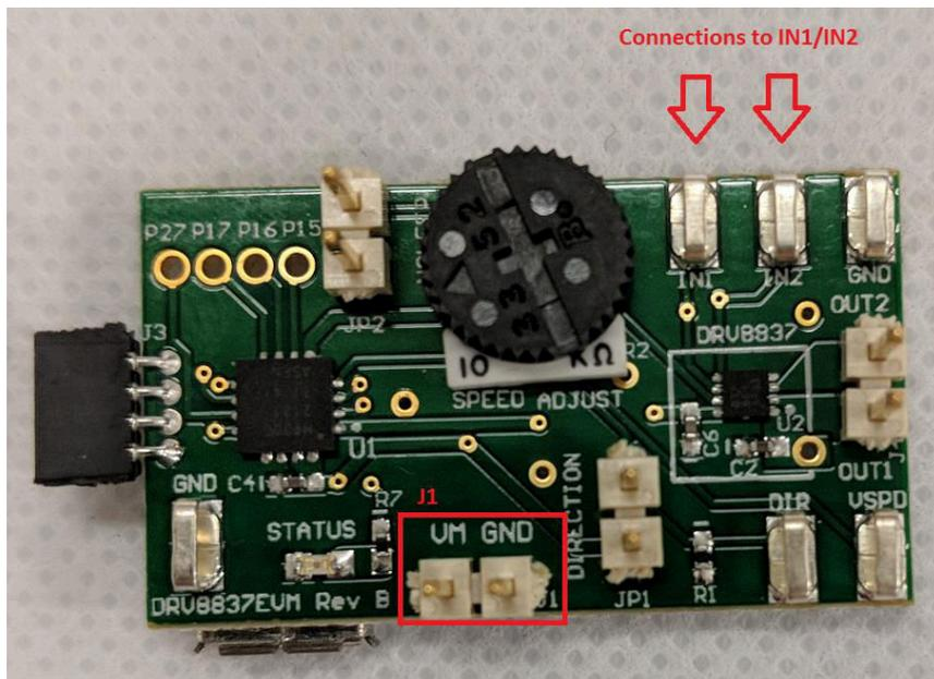
Figure 3-4. J1 and IN1/IN2 Highlighted on Front of DRV8837EVM
