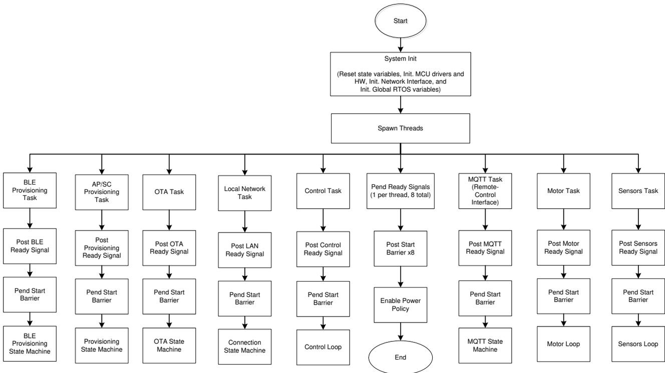
**Figure 2-4. Overall Software Flow Diagram**
