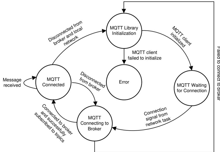
**Figure 2-8. MQTT Thread Main Loop**
