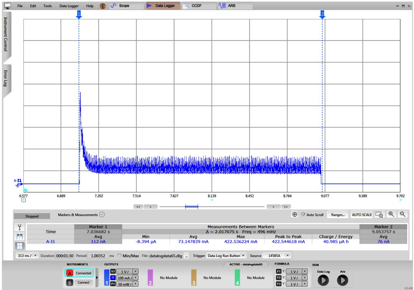
Figure 3-21. DRV8837 Current During Unlock Event
