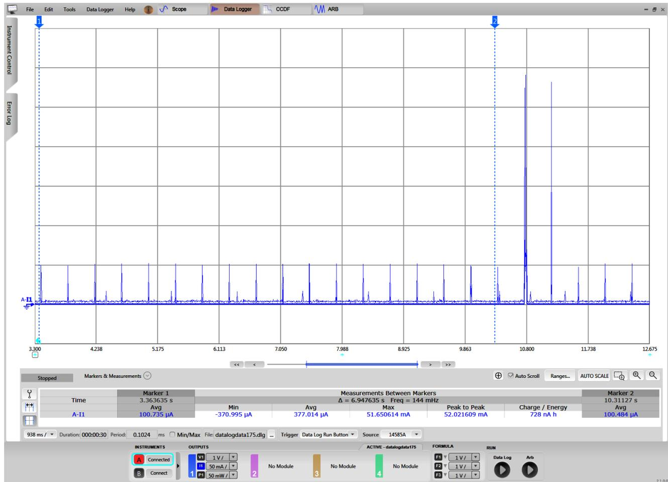
Figure 3-15. CC3220S Current Consumption Versus Time While in Idle Connected Mode With 400-ms LSI
