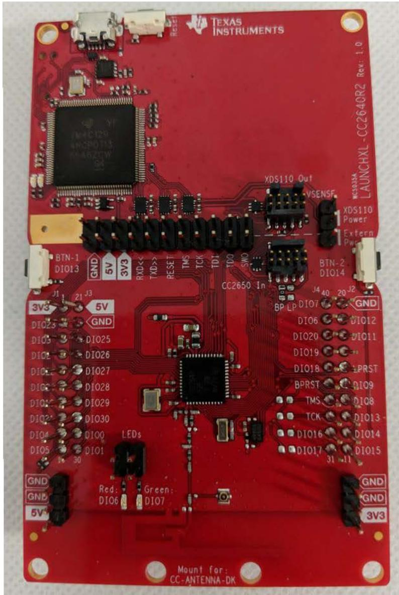
Figure 3-2. CC2640R2F LaunchPad Kit Configuration
