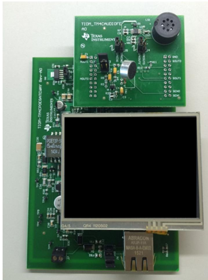
Figure 16. Mounting the LCD Touch Panel
