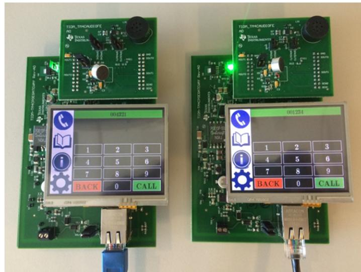
**Figure 34. Board Status After Node Number Configuration**
