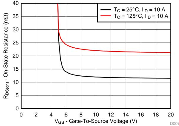
Figure 12. On-State Resistance as a Function of Gate-to-Source Voltage of CSD19537Q3
