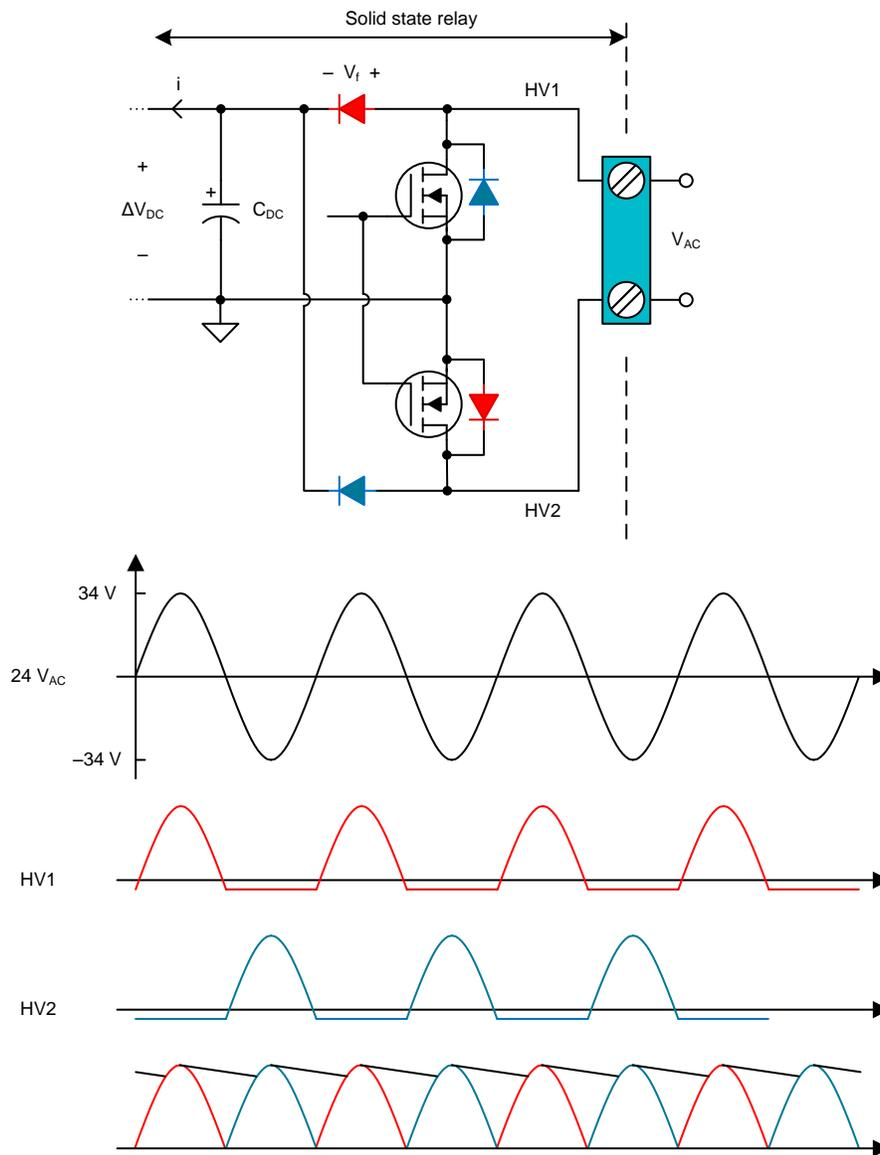
**Figure 11. Full-Wave Rectification Circuitry and Waveforms**
