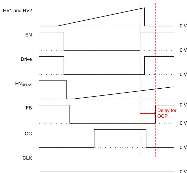
Figure 21. Delay Results for OCP Functionality
