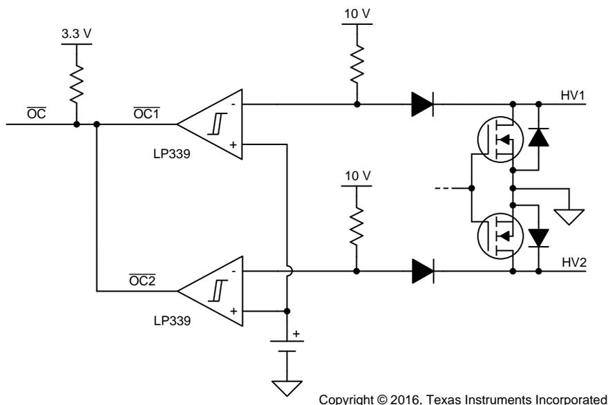
Figure 17. Simplified Schematic of OCP
