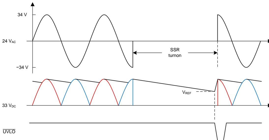
Figure 16. Resulting Waveforms for DC Supply and UVLO When SSR Cycles ON and OFF
