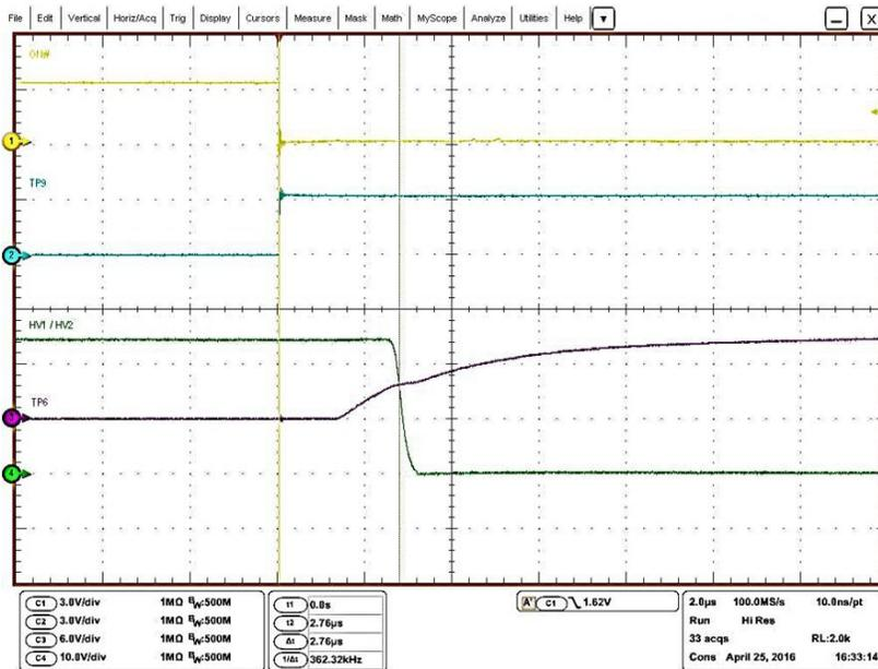
Figure 29. ON Delay Waveforms From Logic Enable Input (Yellow) to TP9 (Blue), TP6 (Purple), and Load of the MOSFETs (Green)
