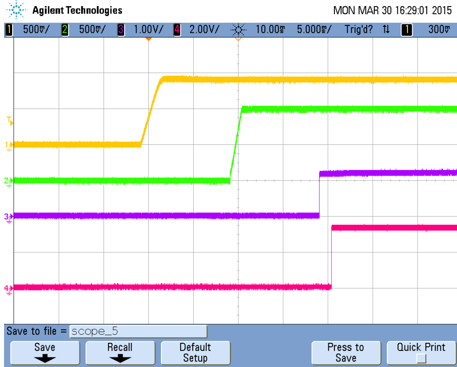
Figure 5 Power up sequence of VCCINT 0.9V, MGTAVCC 1V, MGTAVTT 1.2V, VCCO 3.3V
