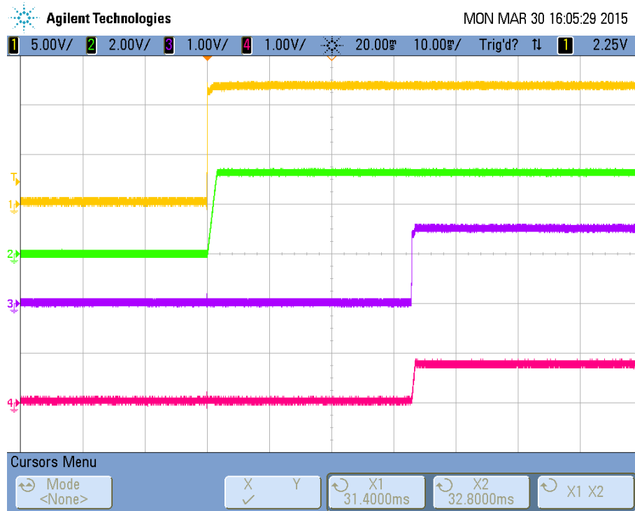
Figure 10 Power up timing of Vin 12V, VAUX 3.3V, VCCO 1.5V, VTT 0.75V
