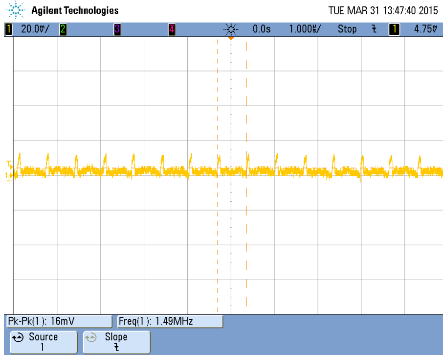
Figure 23 Output ripple of MGTA VCC 1V output at full load, 12Vin
