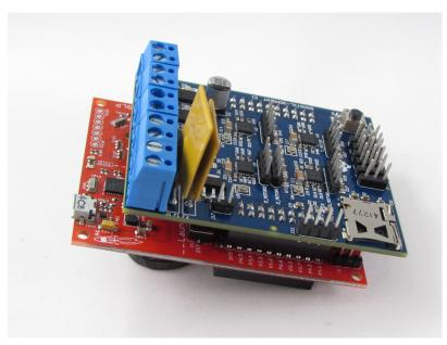
Figure 1: 12V 3D Printer Controller Reference Design
