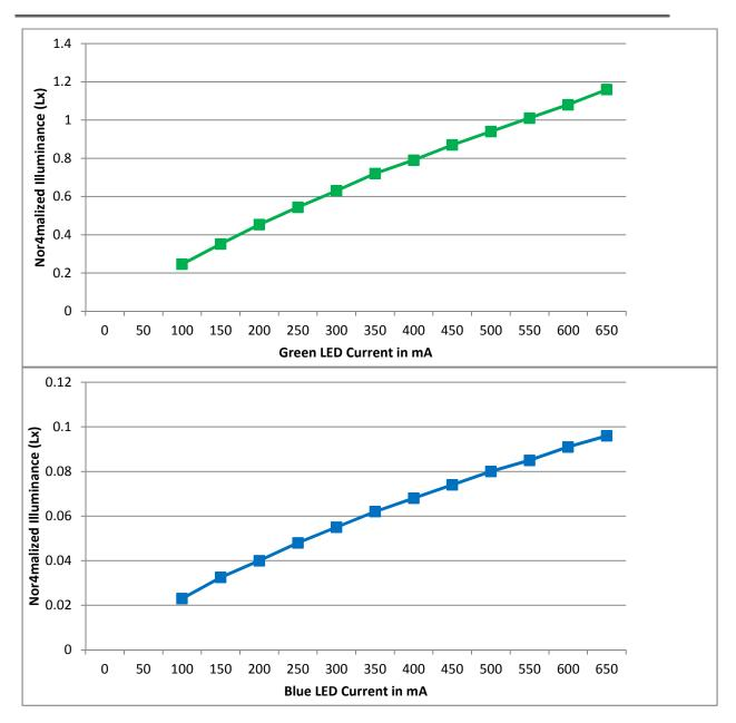
For a typical application current applied to the RGB LEDs is in a specified proportion to achieve a desired white point.
