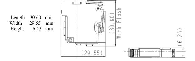
Total volume of the optical engine is: 4-6 cc Weight of the optical engine: 15 gram.
