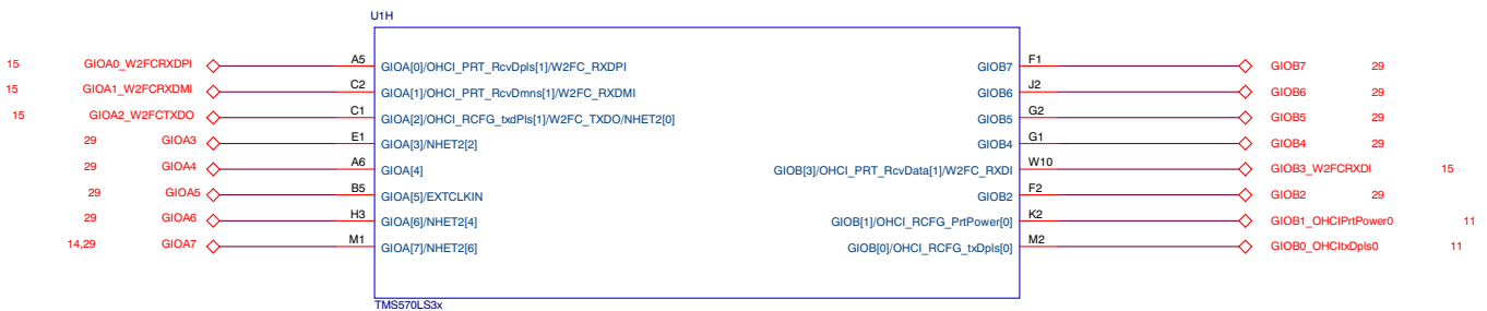
Figure 14. MCU GPIO Schematic
