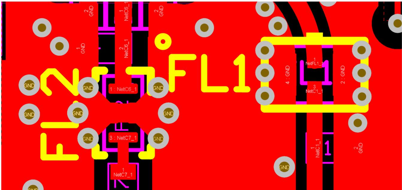
The RF filter must be placed close to the device pin, between the antenna and the device. The RF filter should have a good ground connection to the L2 ground plane. TI recommends adding at least two ground vias near the ground pins to ensure good RF grounding.
