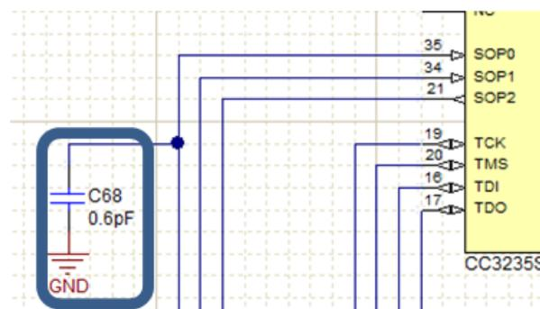
These Capacitor values were selected based on there parasitic effects at higher frequency. These components help filter spurs in the 7-10 GHz band. When selecting capacitors, use either the same capacitors or capacitors with similar parasitics.
