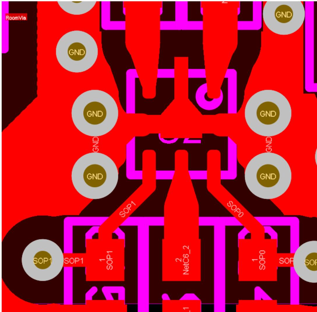
The RF switch should have a good ground connection to the L2 ground plane. TI recommends adding at least two ground vias on both sides ground pad to ensure good RF grounding. Care must be taken in routing the path to the control pins to ensure minimal noise on line
