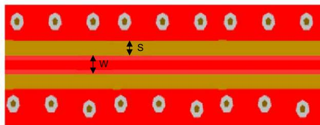
For minimal reflections due to mismatch ensure there is no abrupt change in width of the trace. TI recommends tapering/filleting the trace to the component pads where possible. The RF trace bends must be made with gradual curves, avoid 90-degree bends and sharp corners. Impedance matching networks should also be implemented to ensure continuous 50 ohms impedance. See [Section 4.1.6](#) for more information.
