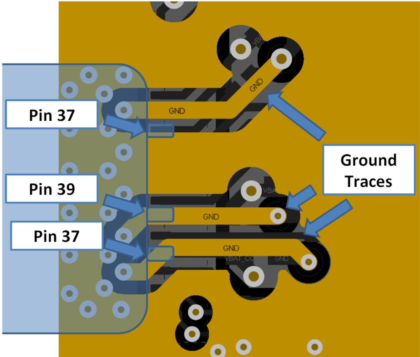
The ground return for the input capacitors are routed on L2 to reduce the EMI and improve the spectral mask. This routing must be strictly followed because it is critical for the overall performance of the device.
