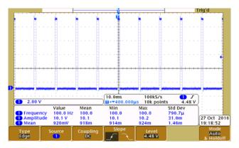
Figure 19. Oscilloscope Measurement of 100 Hz 1-ms pulses
