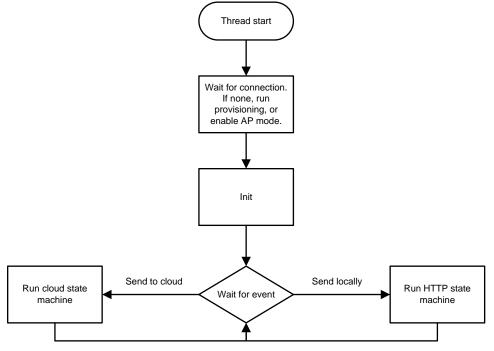
Figure 2. Networking Thread Flow
