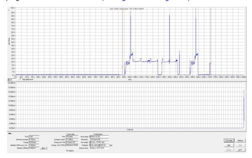
Figure 11. NiDAQ Measurement of Sample CC3100 Program Initialization
