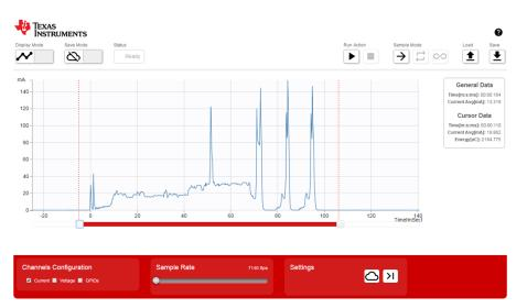
Figure 10. Wireless Scope Measurement of Transceiver Mode
