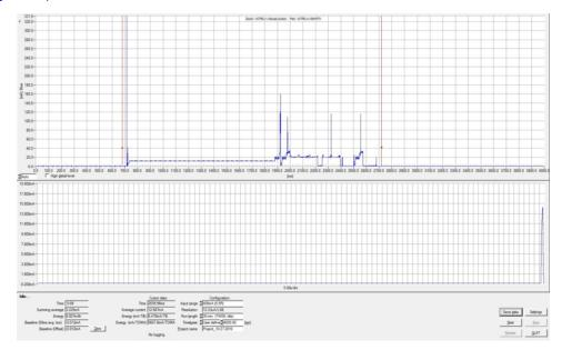
Figure 13. NiDAQ Measurement of CC3100 Wake-Up From Shutdown
