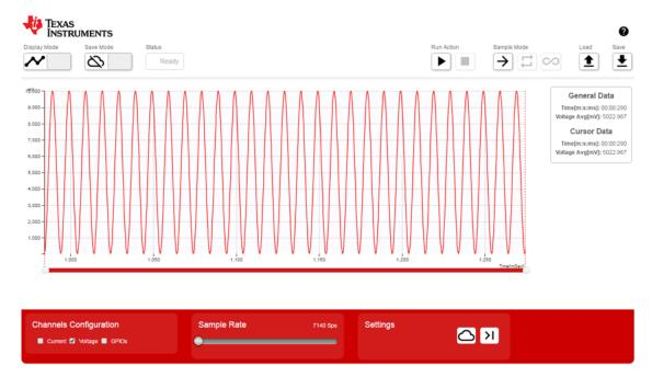
Figure 18. Wireless Scope Measurement of 100-Hz Sine Wave
