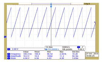
Figure 21. Oscilloscope Measurement of 100-Hz Ramp Wave
