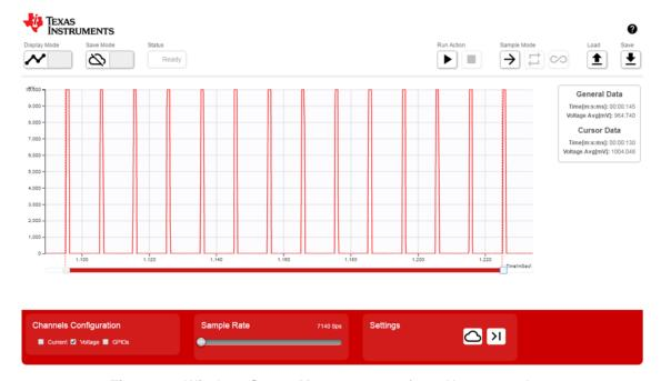
Figure 20. Wireless Scope Measurement of 100 Hz 1-ms pulses
