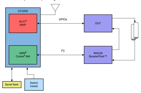
Figure 23. High Level System Block Diagram
