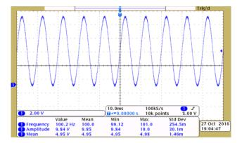
Figure 17. Oscilloscope Measurement of 100-Hz Sine Wave
