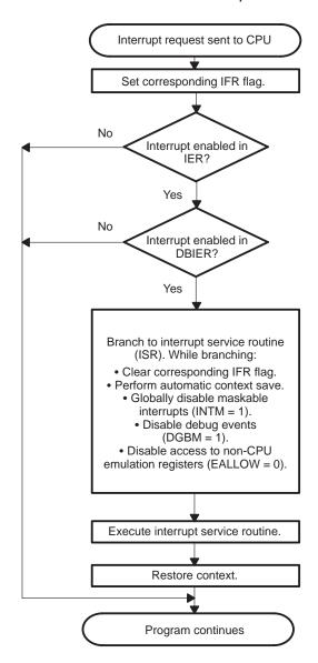
Table 5–4. Steps in the Process Flow for Time-Critical Interrupts
