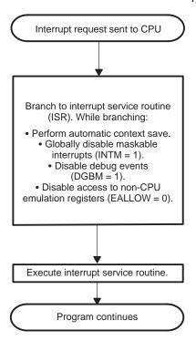
Table 5–5. Steps in the Standard Process Flow for Nonmaskable Interrupts
