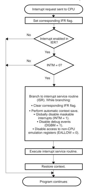
Figure 5–1. Standard Process Flow for Maskable Interrupts
