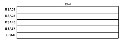
Each buffer start address register is associated with a particular pointer or pointers (see Table 2–5). A buffer start address is only added to the pointer value when the pointer is configured for circular addressing in status register ST2\_55.
