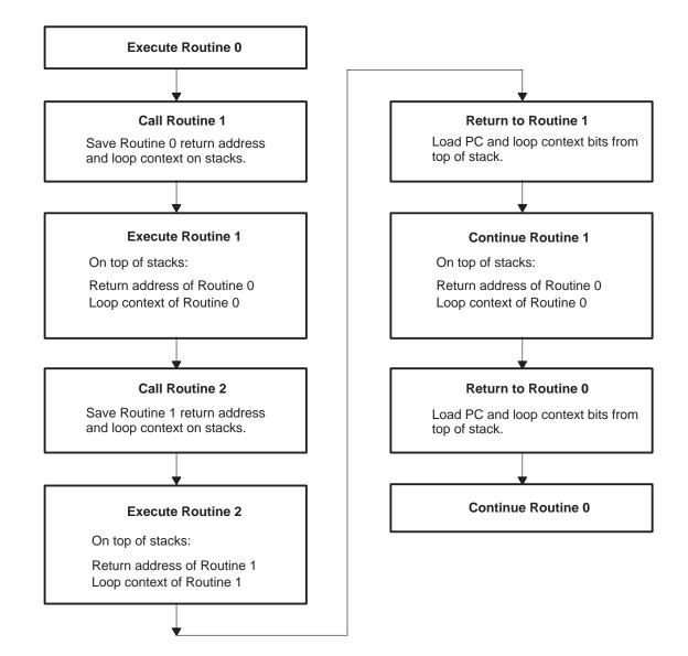
Figure 4–3. Use of RETA and CFCT in Fast-Return Process
