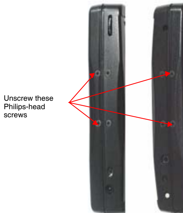
Figure 9–1. Location of Screws for Disassembly
