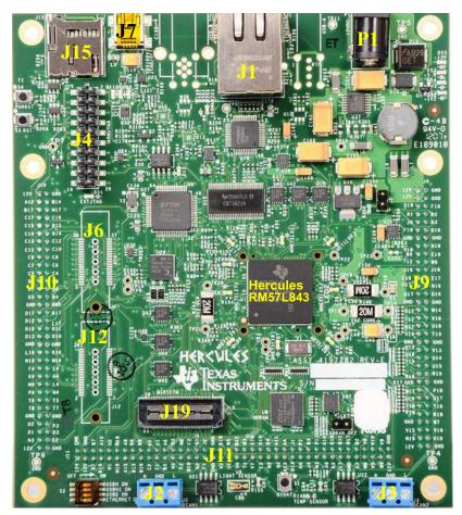
Figure 2-2. Connectors on RM57L HDK
