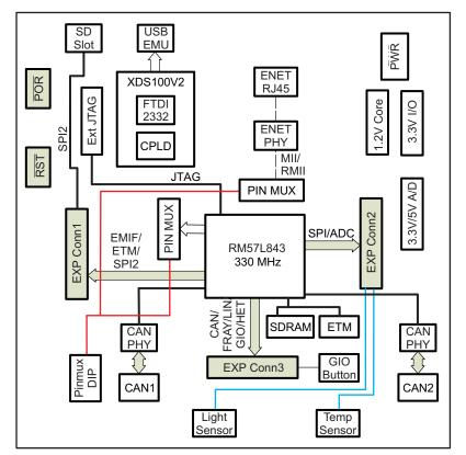
Figure 1-1. RM57L HDK Board Block Diagram
