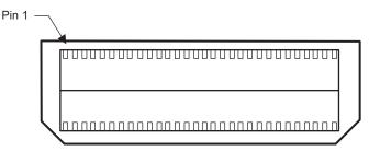
Figure 2-5. J19, 60 Pin MIPI ETM Header
