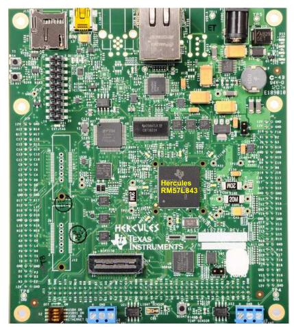
Figure 2-1. RM57L HDK Board, Interfaces Top Side
