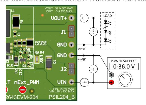
Figure 4-2. VIN and VOUT+ (LED) Connections
