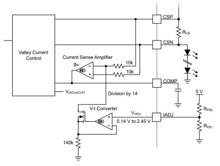
Figure 4-5. Setting IADJ Using On-Board Resistor Divider
