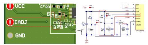
Figure 4-6. IADJ Using Resistor Divider
