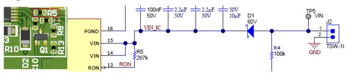
Figure 4-9. Switching Frequency Selection Based on RON (R5)
