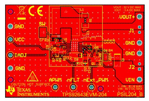
Figure 7-1. Top Layer and Top Overlay (Top View)
