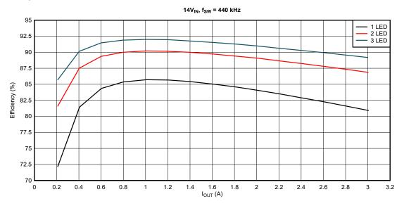
Figure 5-1. Efficiency vs Output Current
