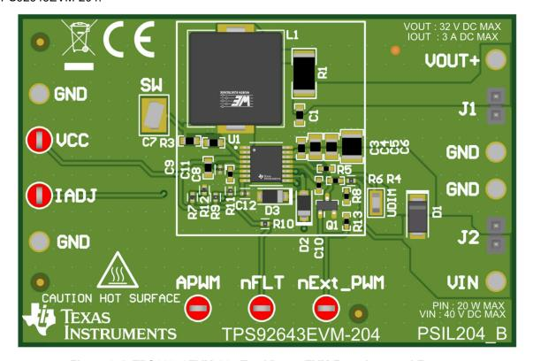
Figure 3-1. TPS92643EVM-204 Top View – EVM Functions and Features
