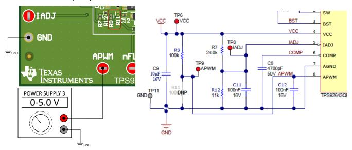
Figure 4-3. Test Setup for APWM
