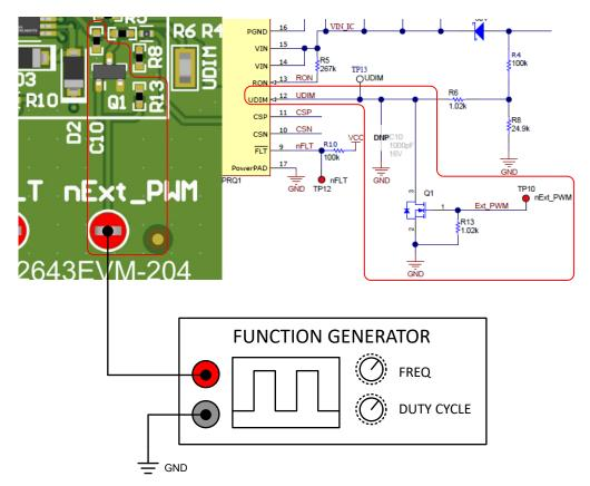
Figure 4-7. PWM Dimming Using nExt\_PWM
