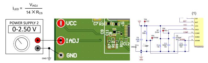
Figure 4-4. IADJ Using External Supply
