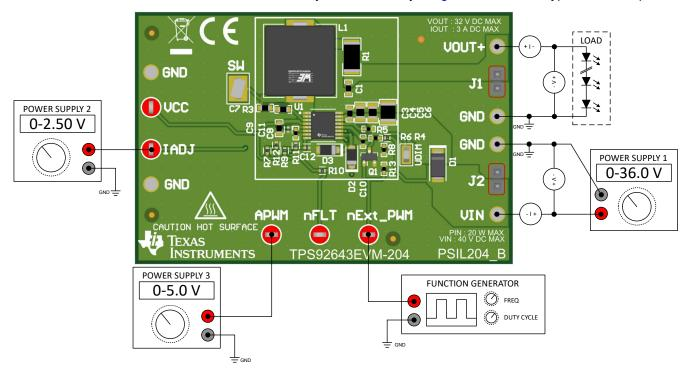
Figure 4-1. TPS92643EVM-204 Typical Test Setup
