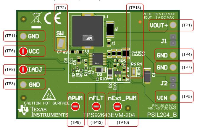
Figure 3-4. TPS92643EVM-204 Test point Numbers and Locations
