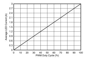
Figure 5-3. Output Current vs PWM Duty Cycle (250 Hz) 14-V Input, 2 LEDs
