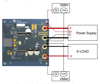
Figure 1. Typical EVM Connection Diagram
