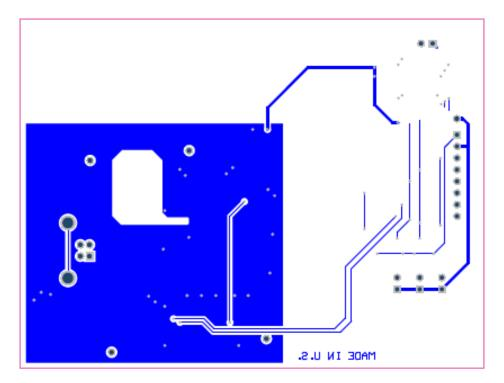
Figure 6: Bottom Layer Routing
