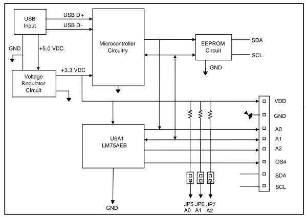
Figure 3: LM75AEB Board Block Diagram
