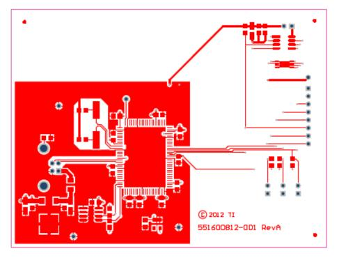
Figure 5: Top Layer Routing
