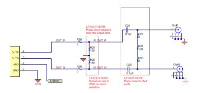
Figure 17. LMK61PD0A2 Output Termination
