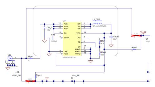
Figure 21. Resistor Configuration to Enable DC-DC
