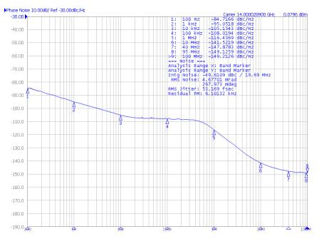
Figure 9. Phase Noise Plot at 14-GHz Output Frequency
