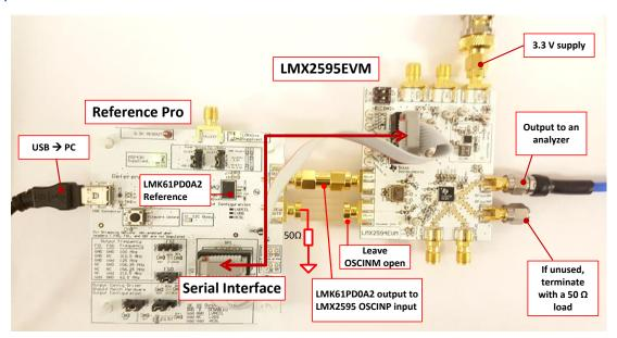
Figure 16. LMX2595EVM Setup With Reference Pro
