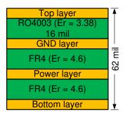
Figure 11. Board Layer Stack-Up
