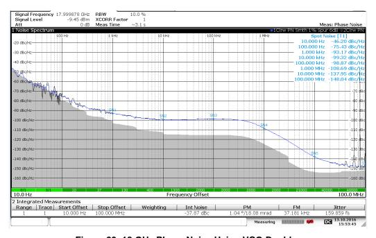
Figure 23. 18 GHz Phase Noise Using VCO Doubler
