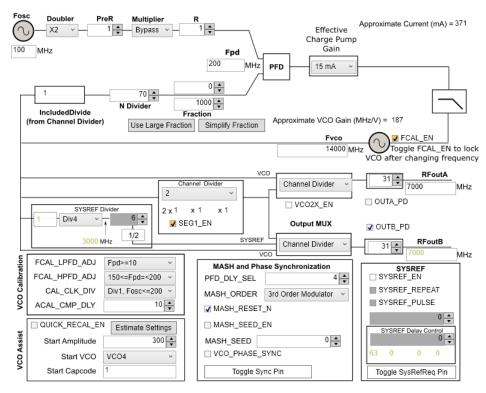
Figure 7. TICS Pro GUI LMX2595 Default Configuration
