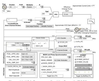
Figure 22. VCO Frequency Doubler Setup in TICSPro
